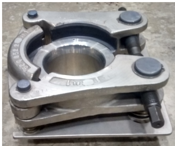
Figure 3-14. Remotely-actuated Grayloc® flange connection system (ORNL photo).
