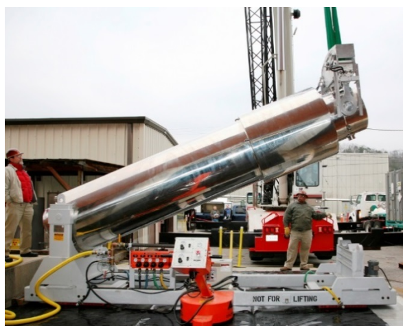
Figure 3-6. LWT® cask being lowered into a horizontal cradle (ORNL photo).
