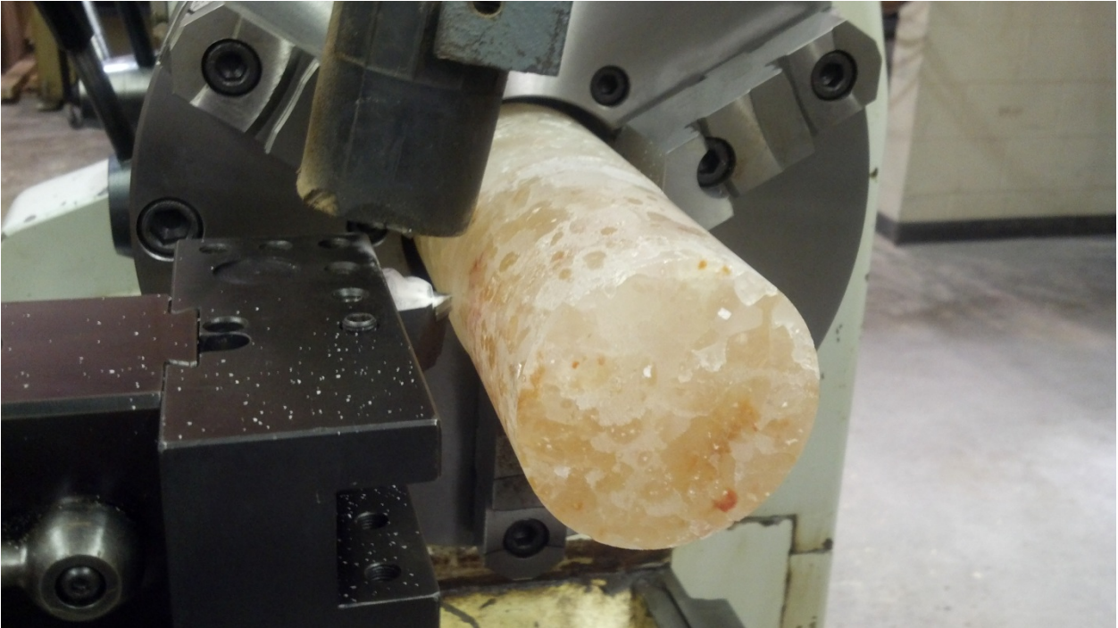
Figure 5. Typical Horizontal Lathe Machining Setup for Preparing Cylindrical Specimens.
