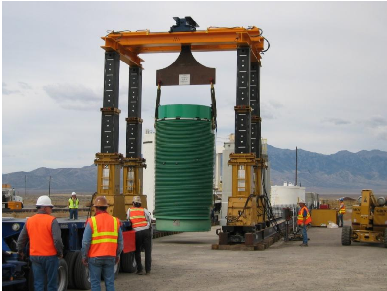
Figure 4-5. CASTOR V/21 as It Is Transported at the Idaho National Laboratory (Photo courtesy of Idaho National Laboratory)
