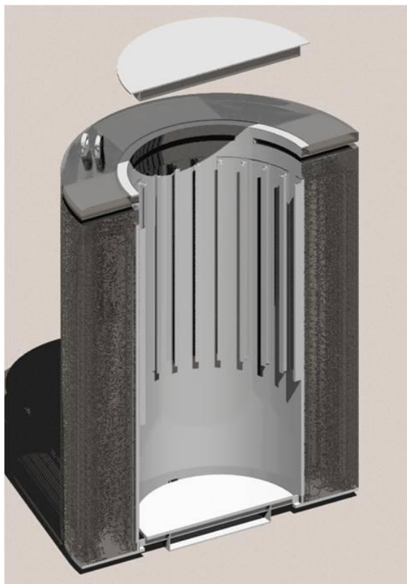
Figure 2-13. NAC MAGNASTOR Basket Inserted in Canister (upper left); MAGNASTOR Vertical Concrete Casks (VCCs) (upper right); Schematic of the MAGNASTOR VCC (bottom). (Images courtesy of NAC International, Inc.; reprinted with permission)
