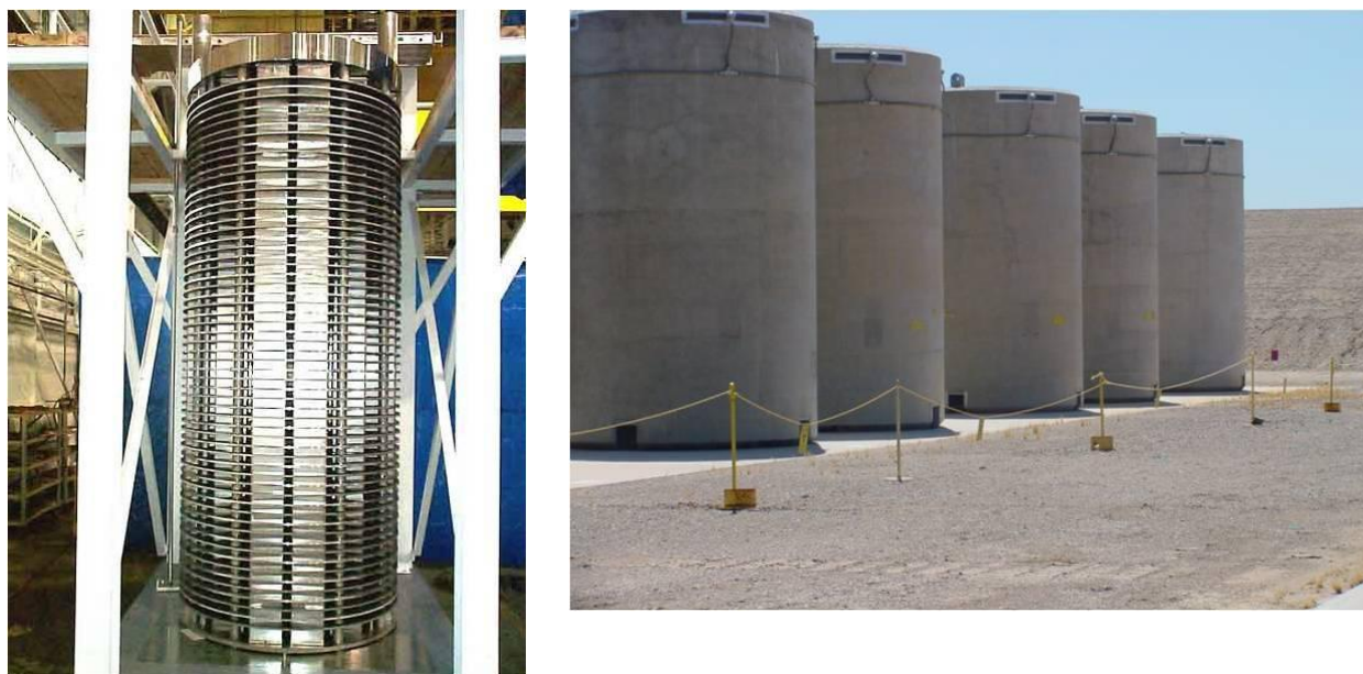
Figure 2-12. NAC UMS Basket (left) and Loaded UMS Systems (right) (Photos courtesy of NAC International, Inc.; reprinted with permission)
