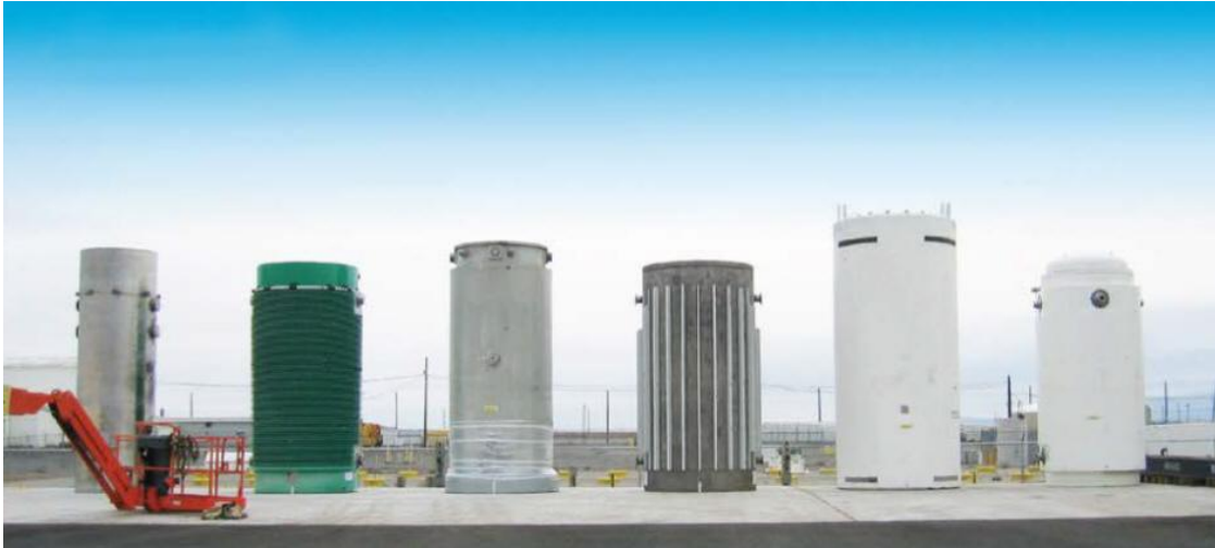
Figure 2-5. Dry Storage Casks at the Idaho National Laboratory INTEC Site Left to right: NAC-I28, CASTOR V/21, REA 2023, MC-10, VSC-17, TN 24P (Photo courtesy of Idaho National Laboratory)
