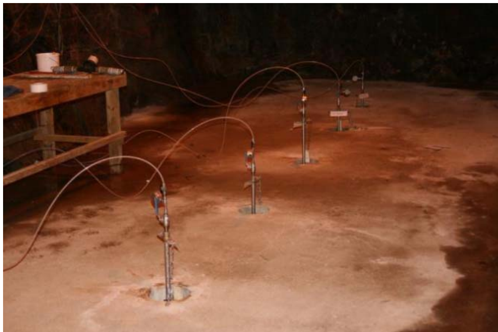
Figure 3-35. BRIE Experiment at Äspö HRL: The test niche and five boreholes (distance 1.5 m) used for initial characterization and selection of BRIE site (SKB, 2011b)
