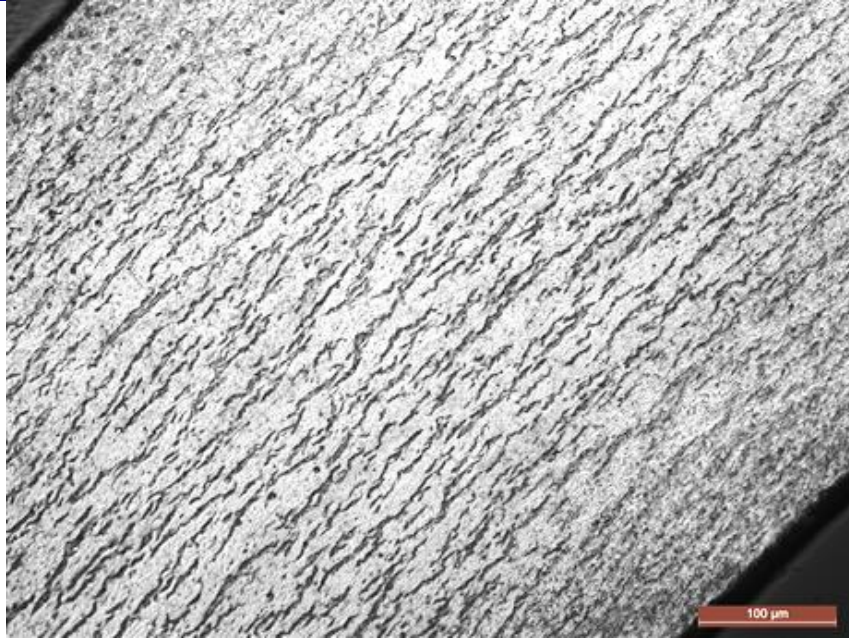
Figure 10. Micrographs showing hydride distributions in hydrogen-charged Zircaloy-4 samples. The average hydrogen content of this location is \approx 610 wppm.
