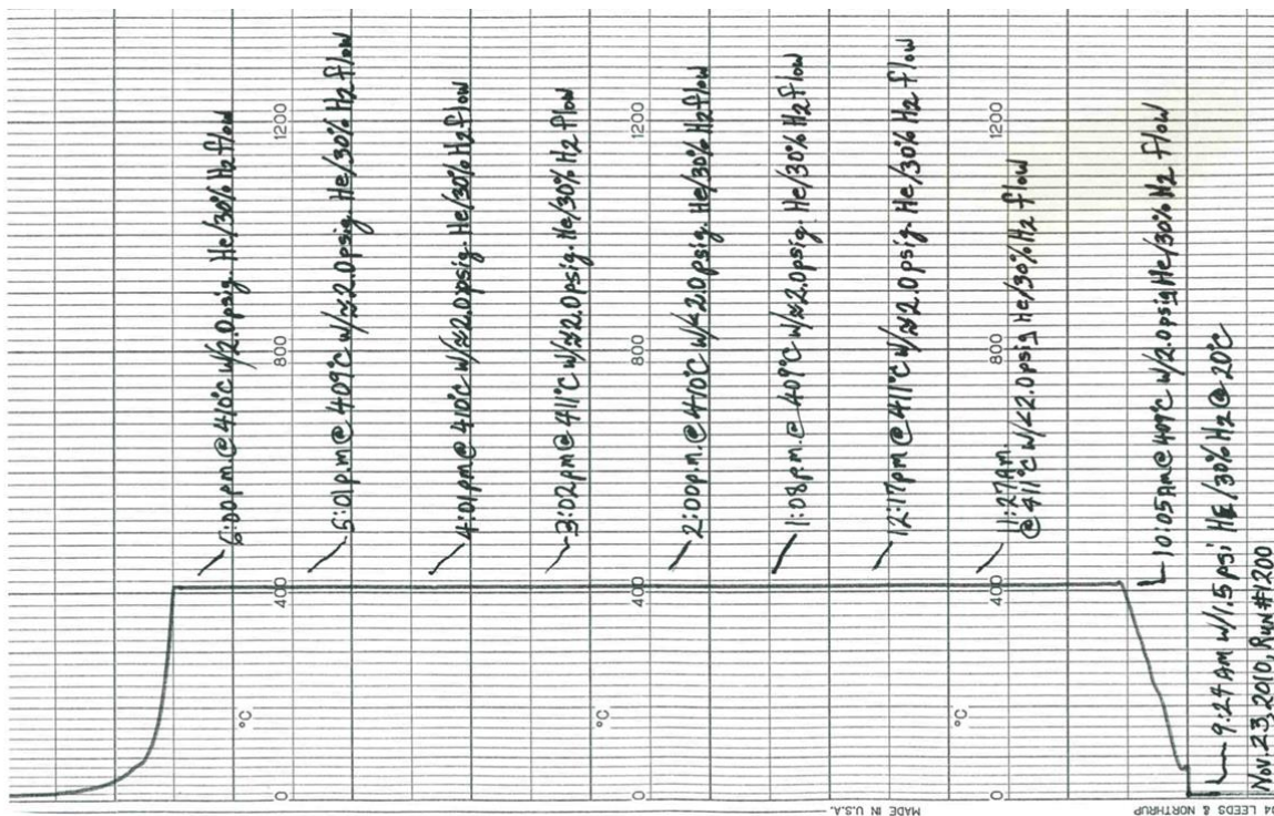
Figure 2. Temperature profile for hydriding cladding materials.
