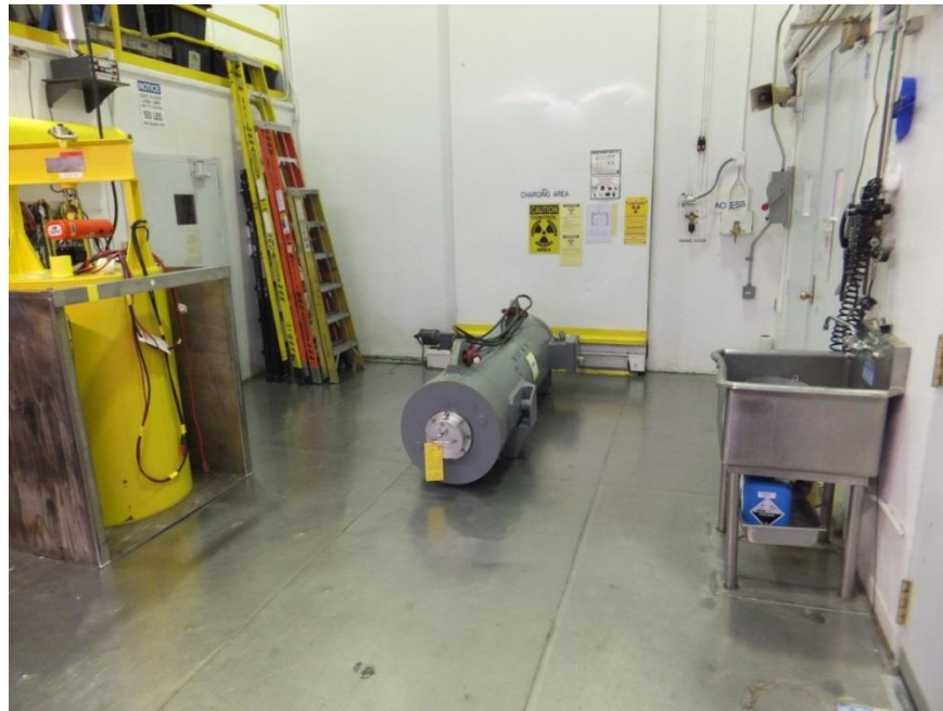
Figure 22. Loop cask for HYCD-1 and HYCD-2 (OD \times L = 2 ft \times 8 ft) at the IFEL.
