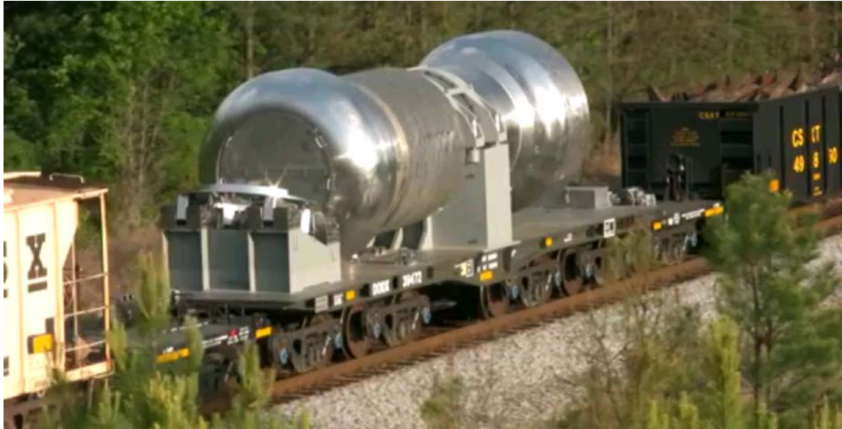
Figure 2.1. Naval UNF Transporter M-290-0001 Cask Car (under commissioning to meet AAR S-2043 [AAR 2003])
