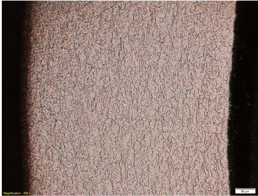
Figure 4.21. Metallographic image of transverse section of the end of sample tube near the Swagelok seal from second autoclave test (200 hours).
