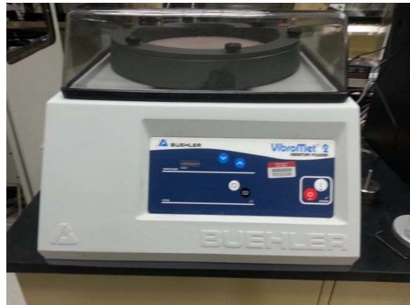
(b) Buehler Vibratory Polisher
