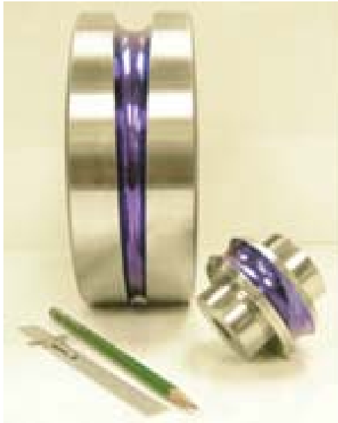
Figure 2.7. Example pilger dies showing the wide variation in design used in commercial zirconium cladding tube production.
