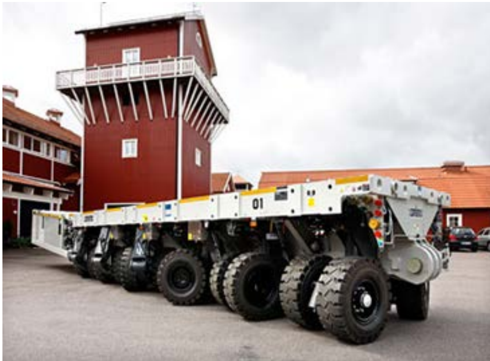
Figure 2.3-1 Diesel Powered Cometto-Built Transporter at Äspö
