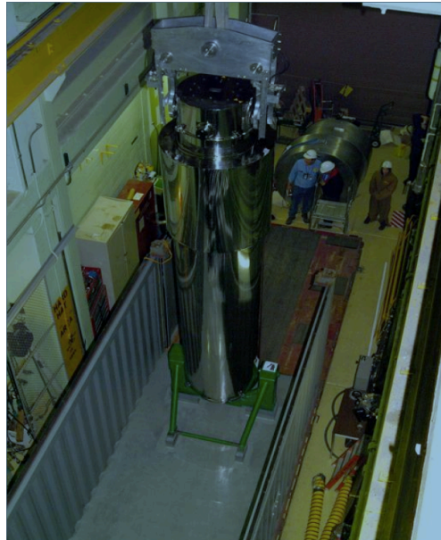
Figure 6-1. A NAC-LWT cask being unloaded in HFEF. The cask is lifted out of the ISO-container and lowered into the cask transfer tunnel and onto the cask transfer cart.
