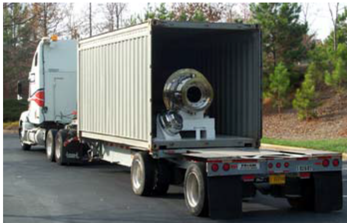
Figure 5-1. NAC-LWT loaded in an ISO-container on a transport trailer demonstrating the transport configuration. The lid is not installed in this image, nor is the end-wall of the ISO-container.
