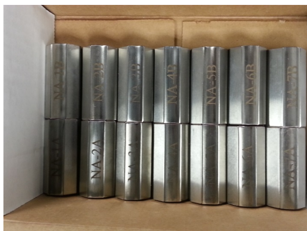
Fig. 16. NA end-caps after laser engraving and spot welding.
