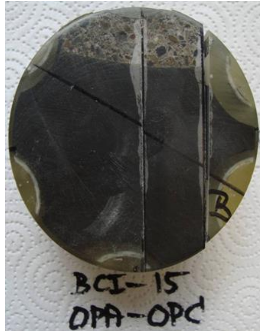
Figure 4.10. OPC concrete – Opalinus Clay sample used in this SANS study. The top part of the sample shows the OPC concrete – Opalinus Clay interface. The lens shaped features surrounding the core are the resin + fiber-glass reinforcements that were inserted parallel to the drilling direction to stabilize the interface region. The photo and core sample were kindly provided by Dr. Urs Mäder.
