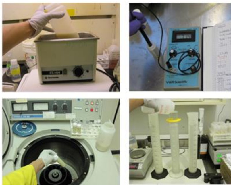
Figure 6-1. Preparation of colloid suspension from FEBEX bentonite brick
