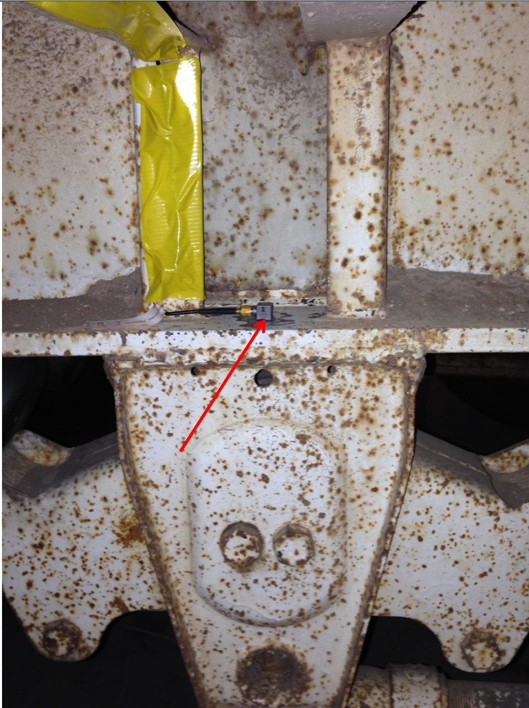
Figure 3.9 Triaxial accelerometer below trailer drop deck above rear axle (see Figures 3.11 and 3.13 and Table 3.1).
