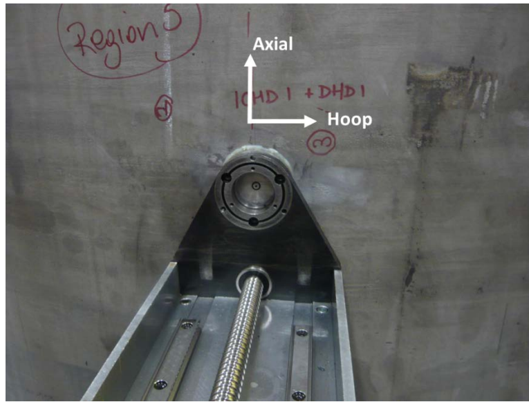
Figure 18: Positioning equipment used to perform DHD measurements of a base metal region (far from any weldments). The orientation of the axial and hoop stresses is indicated on the figure. In the center of the fixture, the hole and EDM overcore can be seen.
