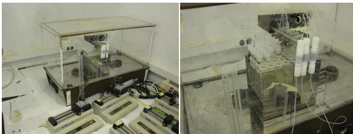
Figure 8-5: Photos of column experiment setup with three 1.5-cm-long columns running in parallel with syringe pumps, tubing, and fraction collector.
