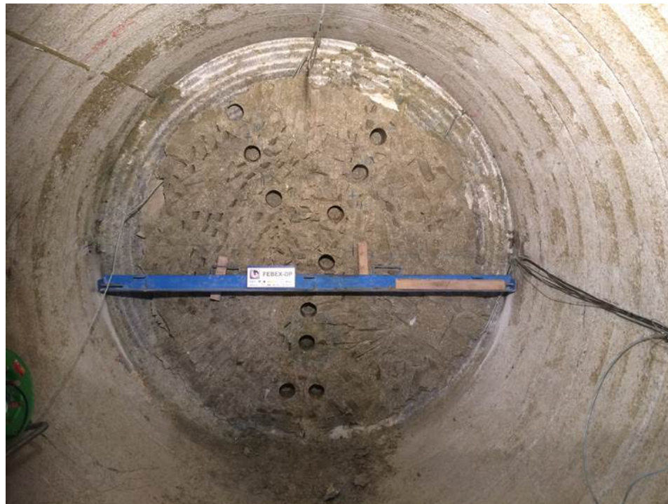
Figure 3.3-12 The front of dismantling section 62 with the core samples taken for microbiological studies, the blue bar prevents the partially detached bentonite from collapsing (Zheng et al., 2016).
