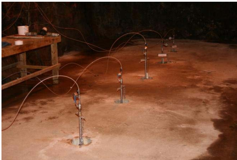
Figure 3.4-3 BRIE Experiment at Äspö HRL: The test niche and five boreholes (distance 1.5 m) used for initial characterization and selection of BRIE site (SKB 2011b).
