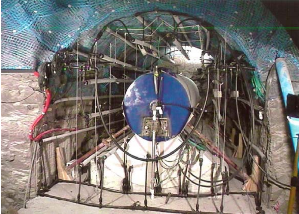
Figure 3.1-14 EB experiment in the construction phase: canister mockup placed on bentonite blocks and hydration pipes (Gens 2016).
