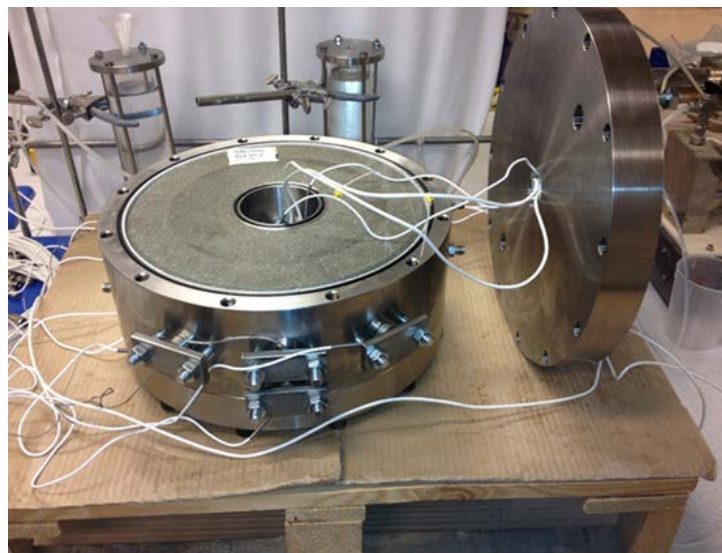
Figure 3.4-8 Top: Schematic view of device geometry used in the large-scale buffer homogenization experiments. Bottom: Photo of the device showing the lid, inlets, and sensors along with bentonite block (Börgesson et al. 2015).
