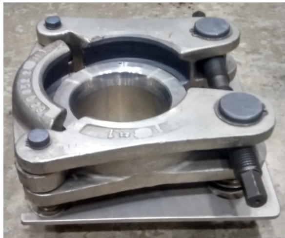
Figure 3-12. Remotely-actuated Grayloc® flange connection system (ORNL photo).
