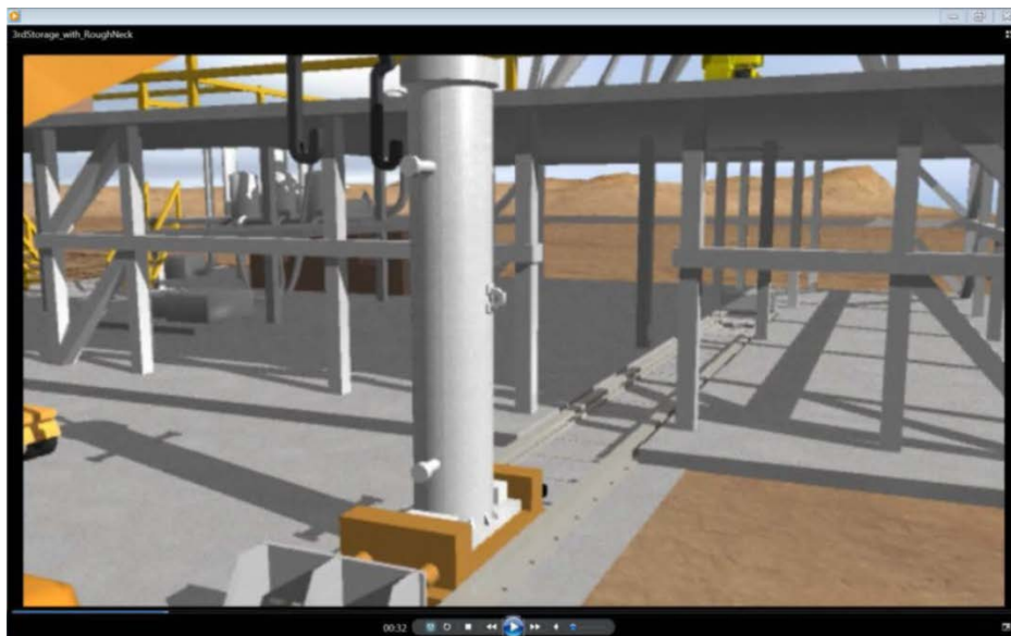
Figure 2-11. Visualization of transportation/transfer cask mounted on transfer carrier, on a track under the rig floor, leading to the wellhead.
