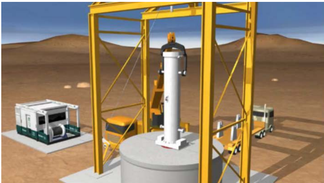
Figure 2-12. Schematic of wellhead shield, top plate, crane, transfer cask in position for waste emplacement, headframe, and wireline winch (not to scale).
