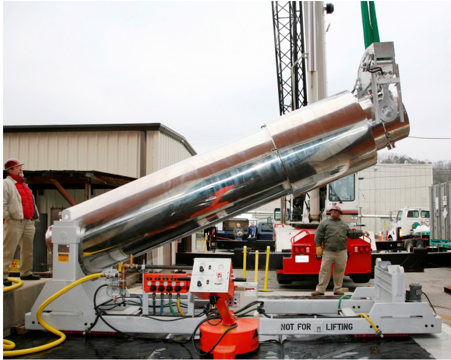
Figure 3-4. LWT cask being lowered into a horizontal cradle (ORNL photo).
