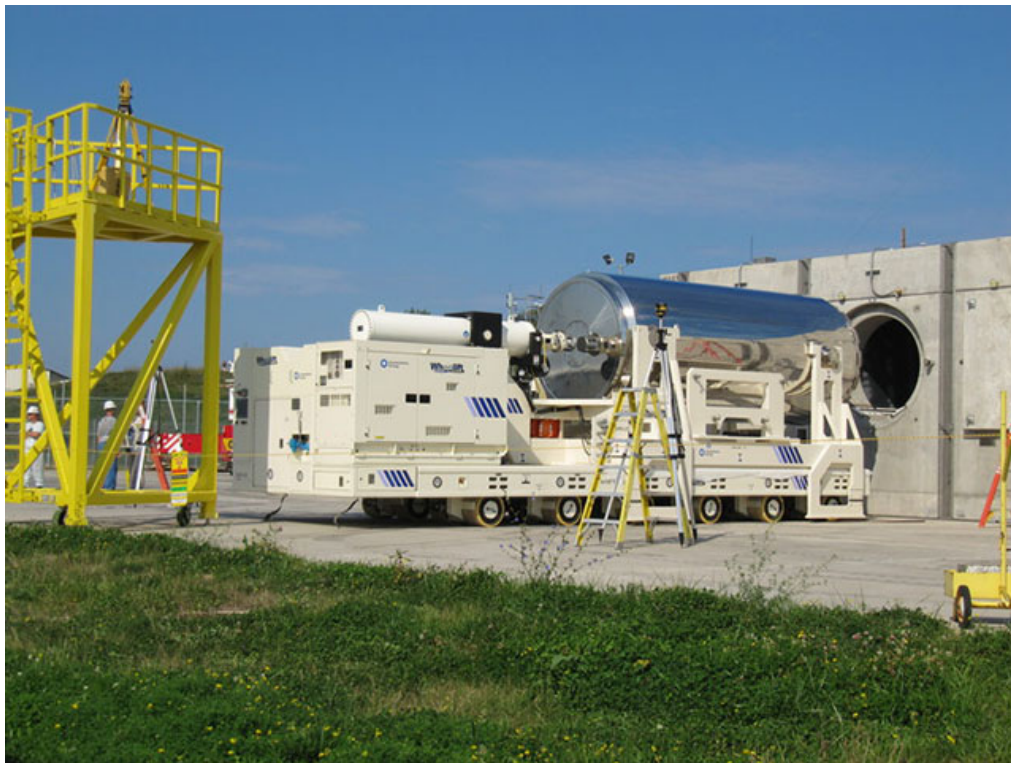
Figure 2-13. NUHOMS® dry storage system with transfer cask, getting in position to push a loaded waste canister into the storage vault on the right ( www.wheelift.com ).
