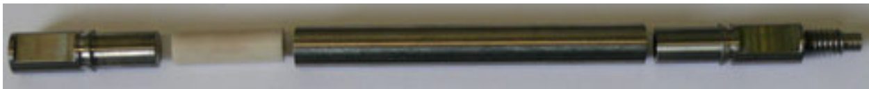
Figure 2: Rodlet components: bottom end fixture, zirconia pellet, cladding segment, and top end fixture.
