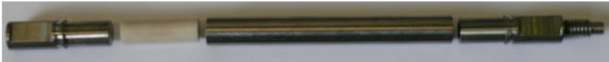
Figure 7: Rodlet bottom end fixture, zirconia pellet, cladding segment, and top end fixture.
