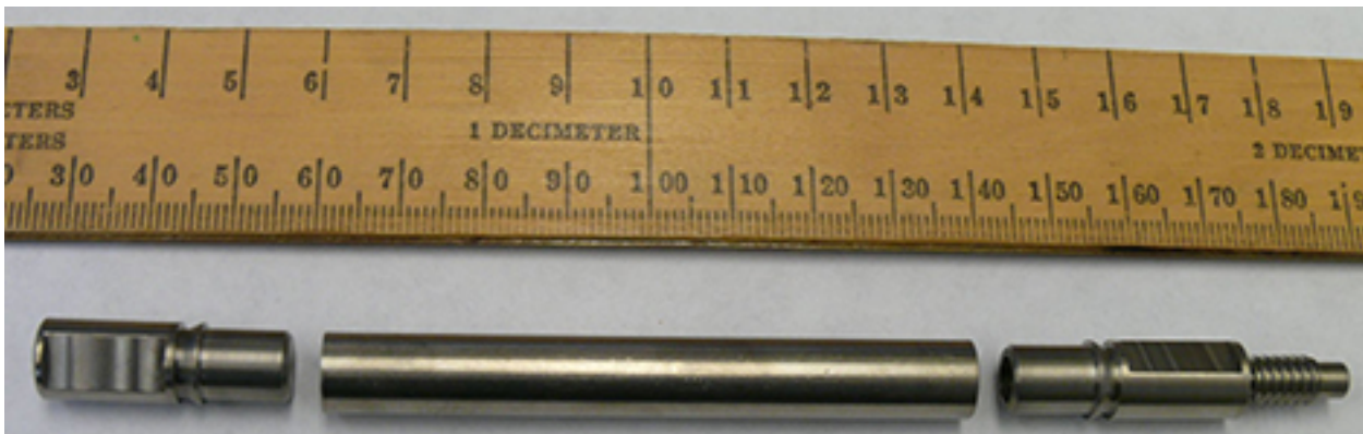
Figure 8: Rodlet bottom end fixture (redesigned), cladding segment, and top end fixture (redesigned).
