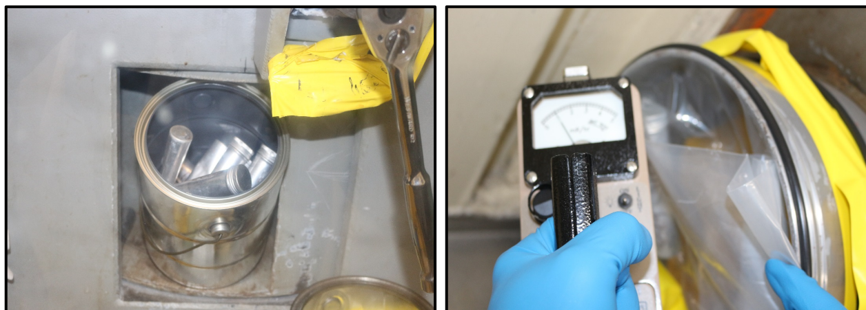
Figure 8. Defueled Cladding Segments in Aluminum Containers Awaiting Shipment to ANL (left) and Contact Dose Rate Measurement on a Single Container (right).
