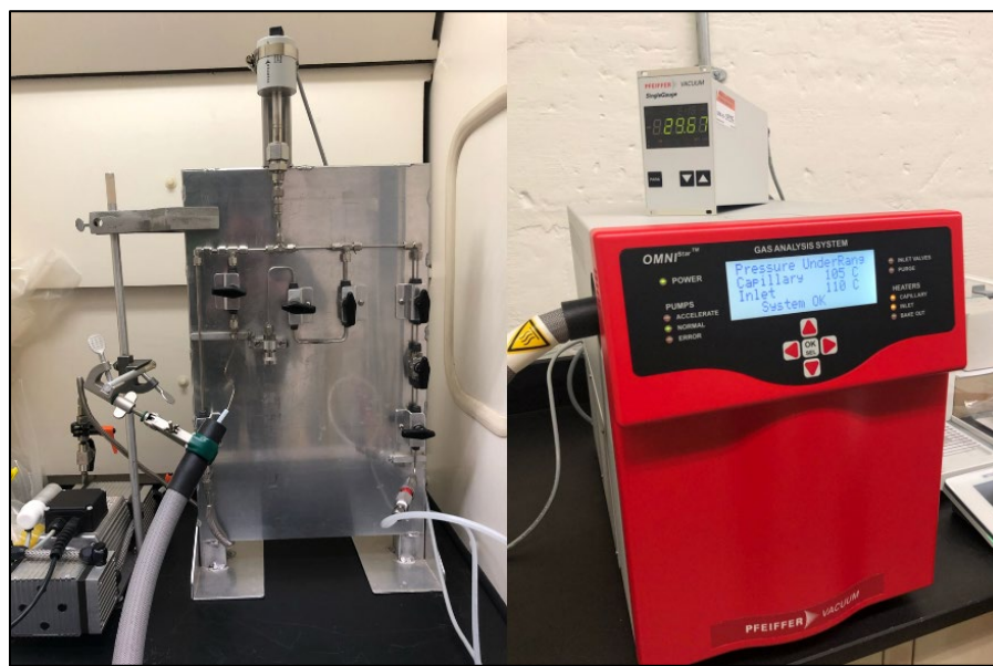
Figure 28. The Sample Inlet Manifold (left) Coupled to an OmniStar GSD 320 Gas Analysis System (RCA) (right).
