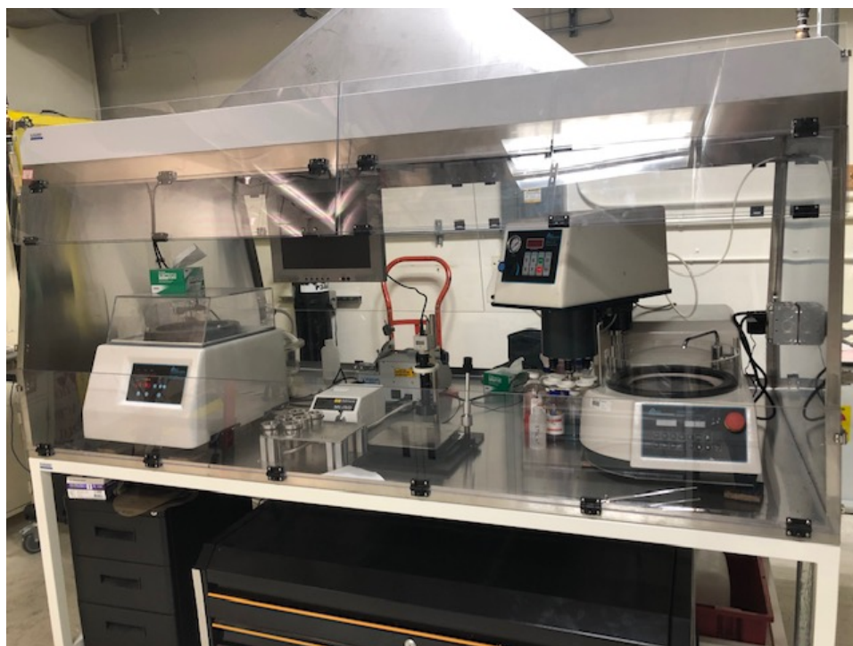
Figure 5-2. Vibratory Polisher and Multistage Polisher
