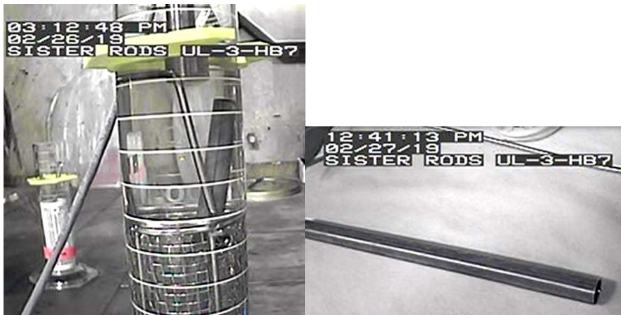
Figure 3-9. Leached and Cleaned Sample UL-3-1
