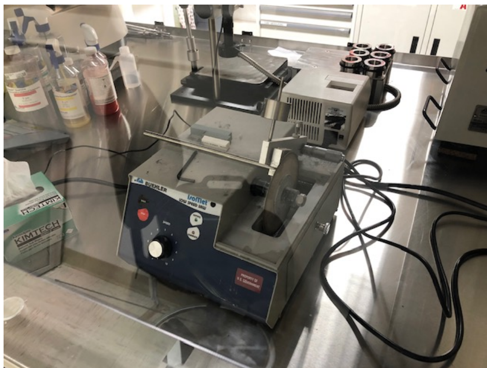
Figure 5-1. Isomet Low-Speed Saw
