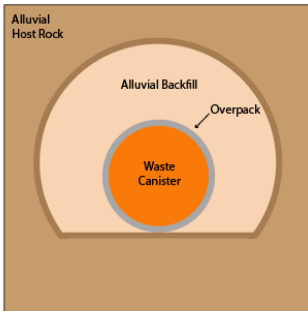
Figure 4-1. Schematic cross-section view of drift for disposal of waste packages in an unsaturated alluvial repository.
