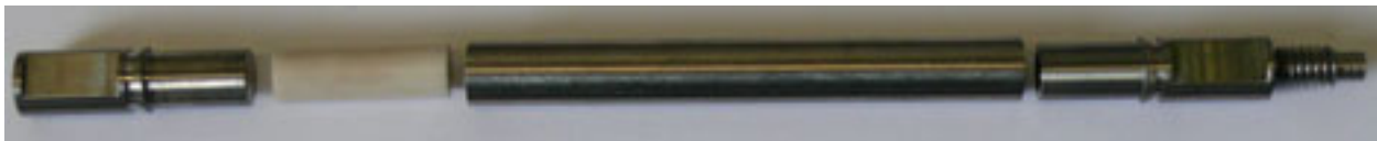
Figure 4: Rodlet bottom end fixture, zirconia pellet, cladding segment, and top end fixture.
