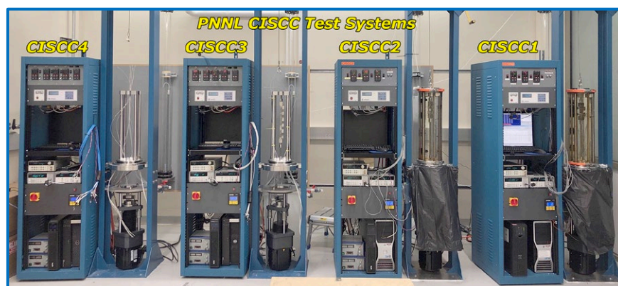
Figure 13. All four PNNL CISCC test systems. CISCC3 and CISCC4 were partially constructed at the time of this photo but are now complete.
