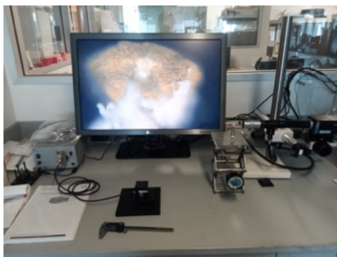
Figure 7-3. Benchtop experiment set-up with display showing a single quartz grain, ~200 microns in diameter, on top of the sample holder
