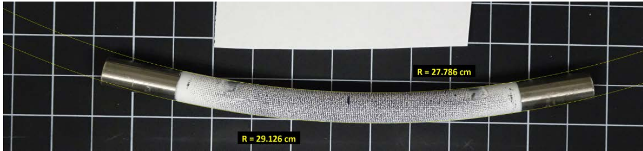
Figure 6-25. Radius of Curvature Measurement on an Unloaded Length of Tubing that Underwent Four-Point Bend Testing. The measurement was made using ImageJ software and the image taken on an inspection microscope.
