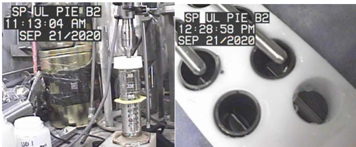
Figure 4-9. Final Rinse of 11 Samples of 1/2 in. Cladding from Rod UL.
