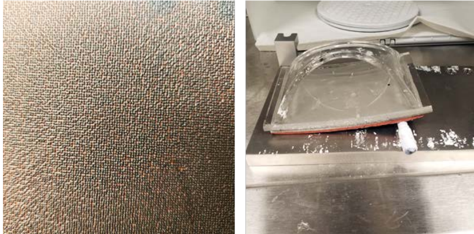
Figure 6-14. Sample Speckle Stamp (left) Being Applied to a Sample (right).
