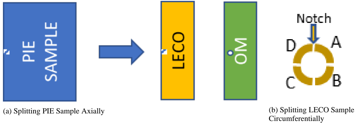
Figure 5-4. Cutting PIE Sample (a) Axially and (b) Circumferentially.
