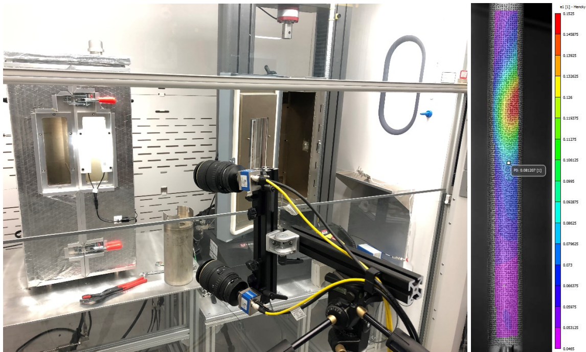
Figure 6-18. DIC System Configured for Burst Testing (left) and Burst Sample Overlaid with Strain Map before Burst (right).
