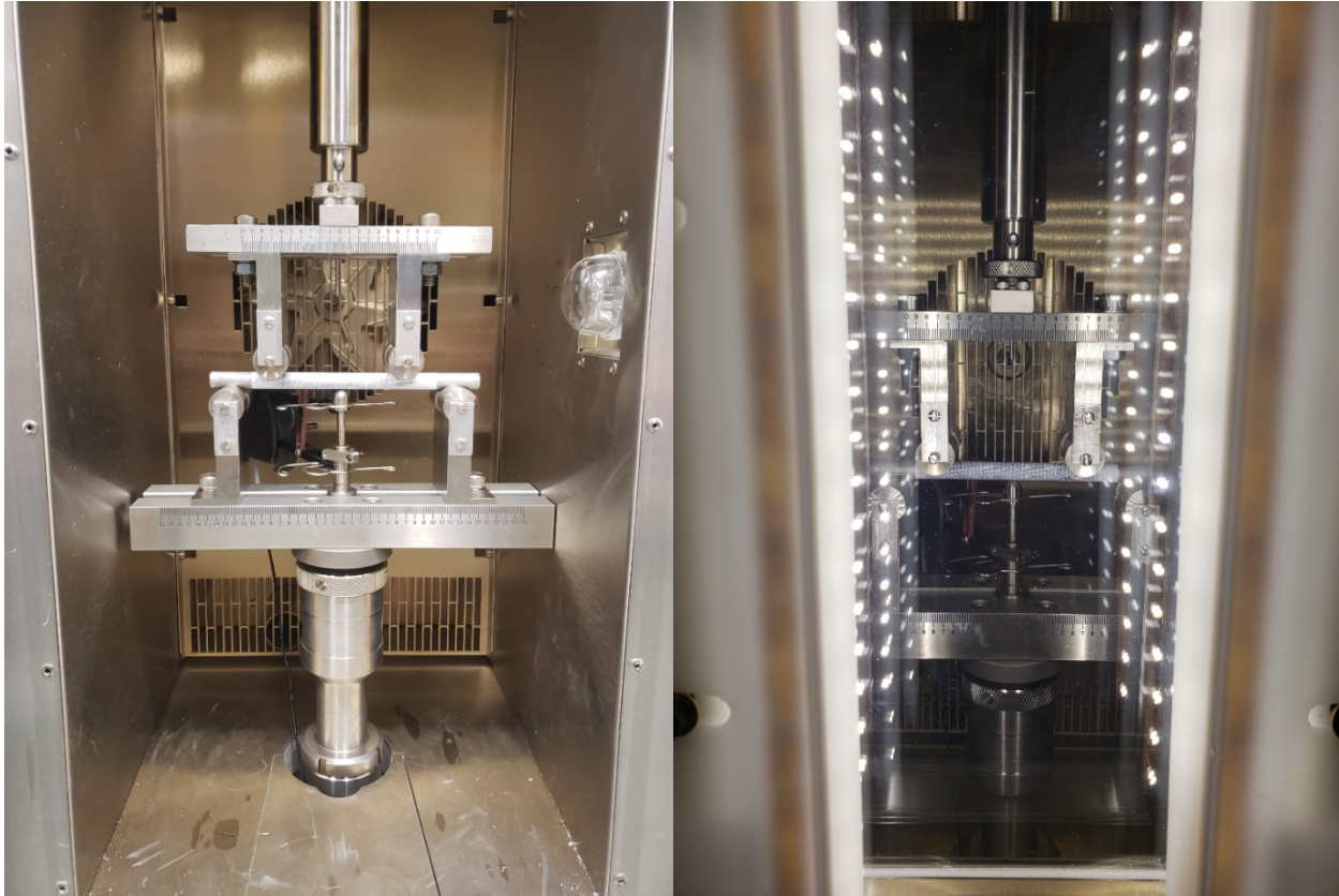
Figure 6-11. Four-Point Bend Fixture Configuration Inside Environmental Chamber.
