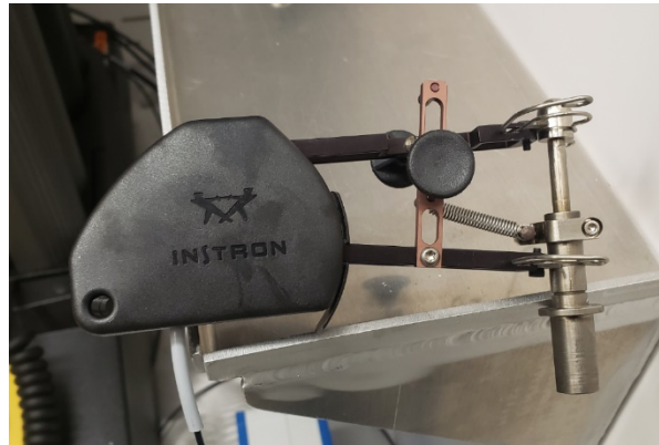
Figure 6-10. Deflectometer Attached to Extensometer Used on Four-Point Bend Fixture.
