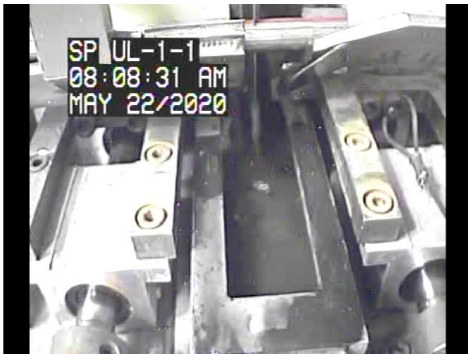
Figure 3-4. Sectioning Saw Water Basin used to Wet the Cutting Blade and Collect Cutting Fines.
