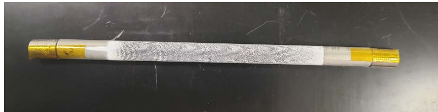
Figure 6-21. Axial Tensile Sample with End Plugs Installed.
