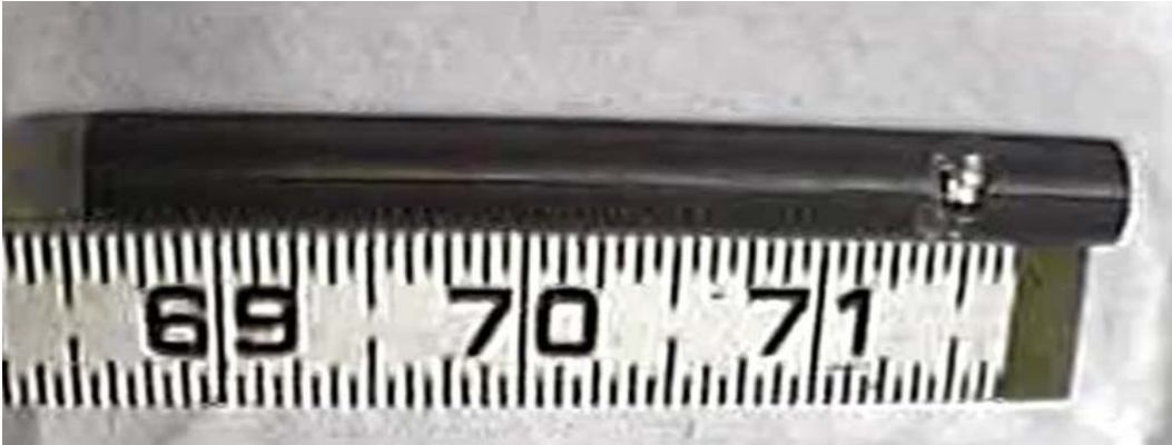
(a) Sample FK-4-1 in Hot Cell After Dissolution of Fuel. Puncture location visible towards left end of sample.
