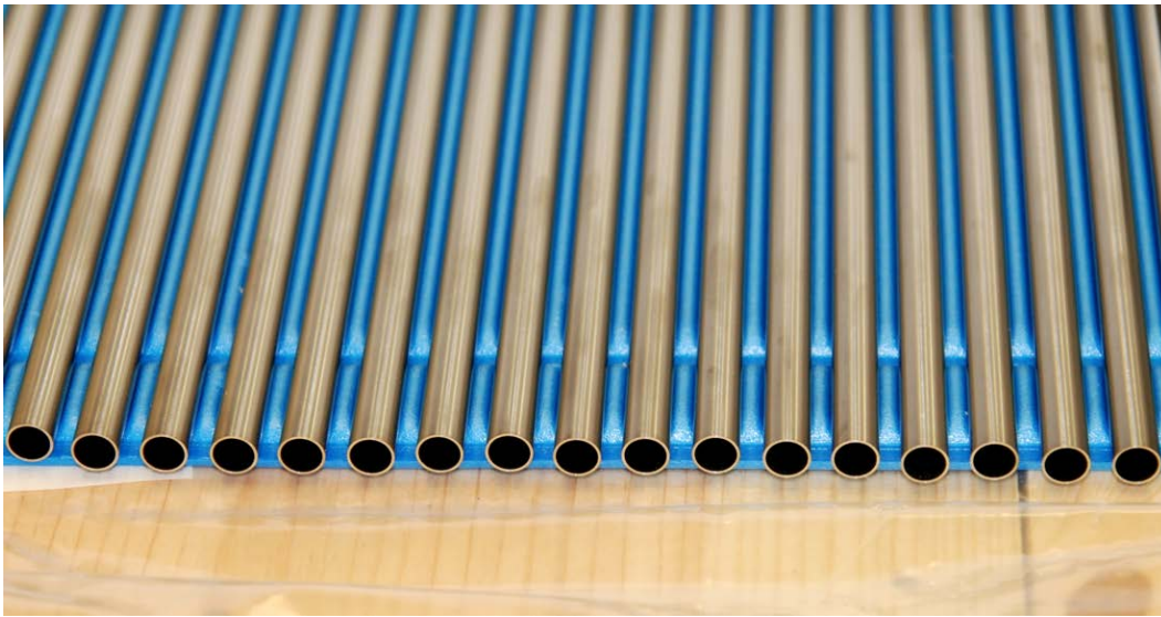
Figure 6-26. Procured As-Manufactured Cladding. (Shimskey et al. 2014)
