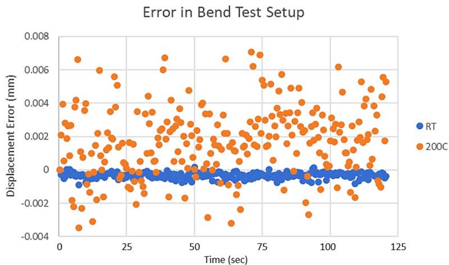
Figure 6-30. DIC Strain Error vs. Time for Four-Point Bend Tests at RT and 200°C.
