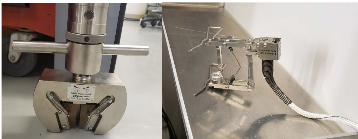
Figure 6-6. Wedge Grip (left) and High-Temperature Extensometer (right) Used in Axial Tensile Tests.
