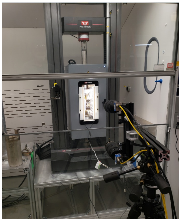
Figure 6-5. Electromechanical Load Frame with Convection Oven and Video Image System.
