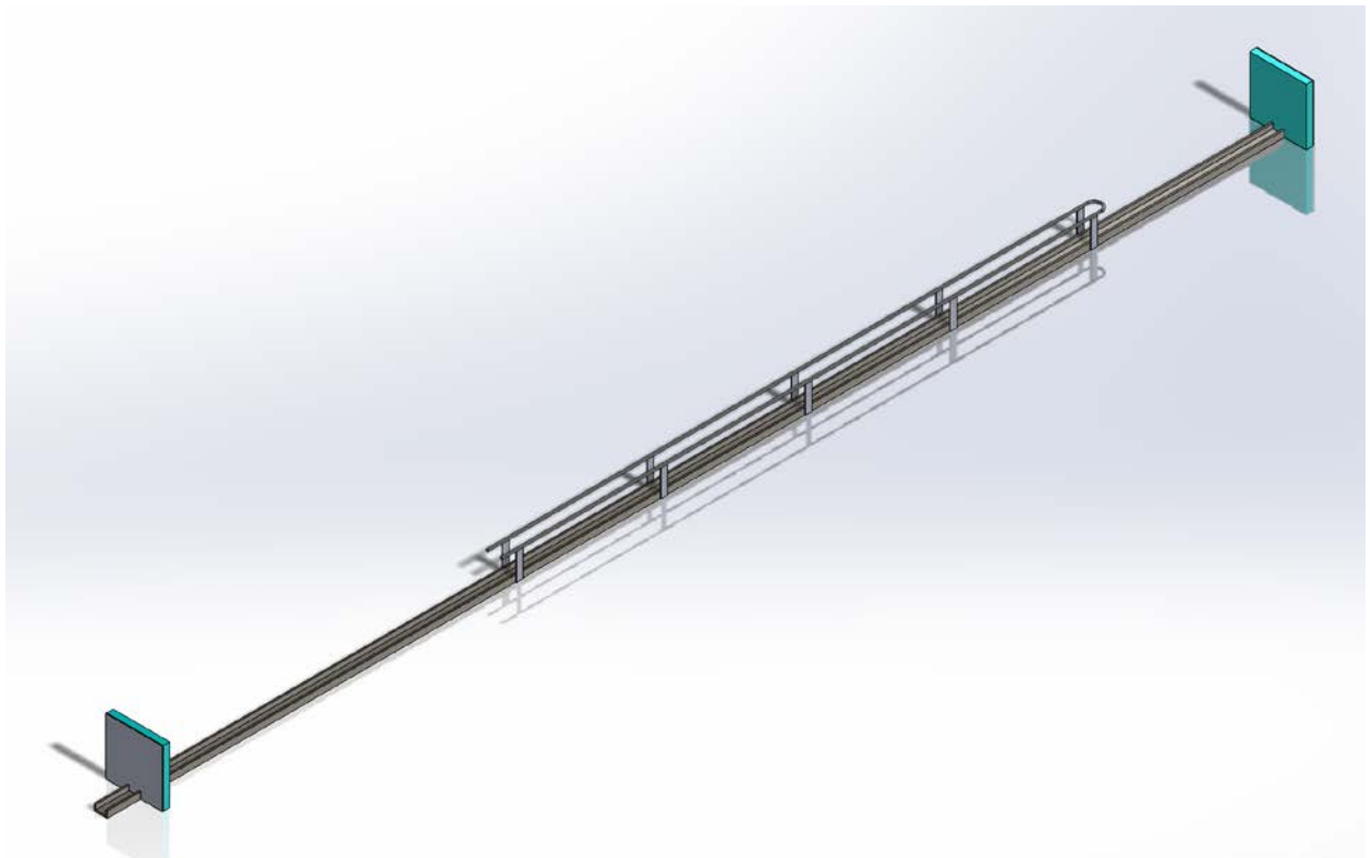
Figure 2-12. CAD Geometry for Electrical Heater Assemblies
