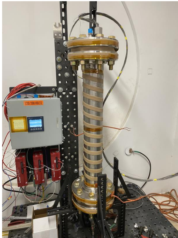
Figure 2-4 Photo of the pressure vessel used for the 5×5 DDA testing. Flexible heaters were wrapped around the pressure vessel to provide simulated decay heat.
