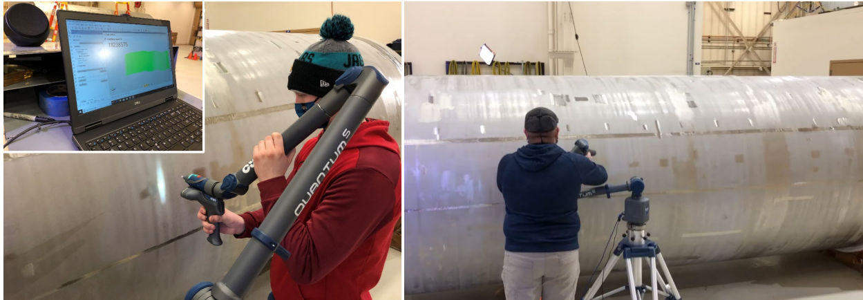
Figure 3.2 Images showing the non-contact laser scanning in progress using an 8-axis Quantum S coordinate measuring machine for position data.
