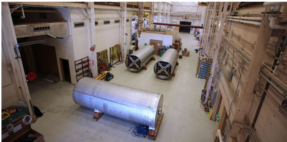
Figure 1.3 Three 32PTH2 spent fuel canisters inside of Sandia’s Building 6630 south high bay.
