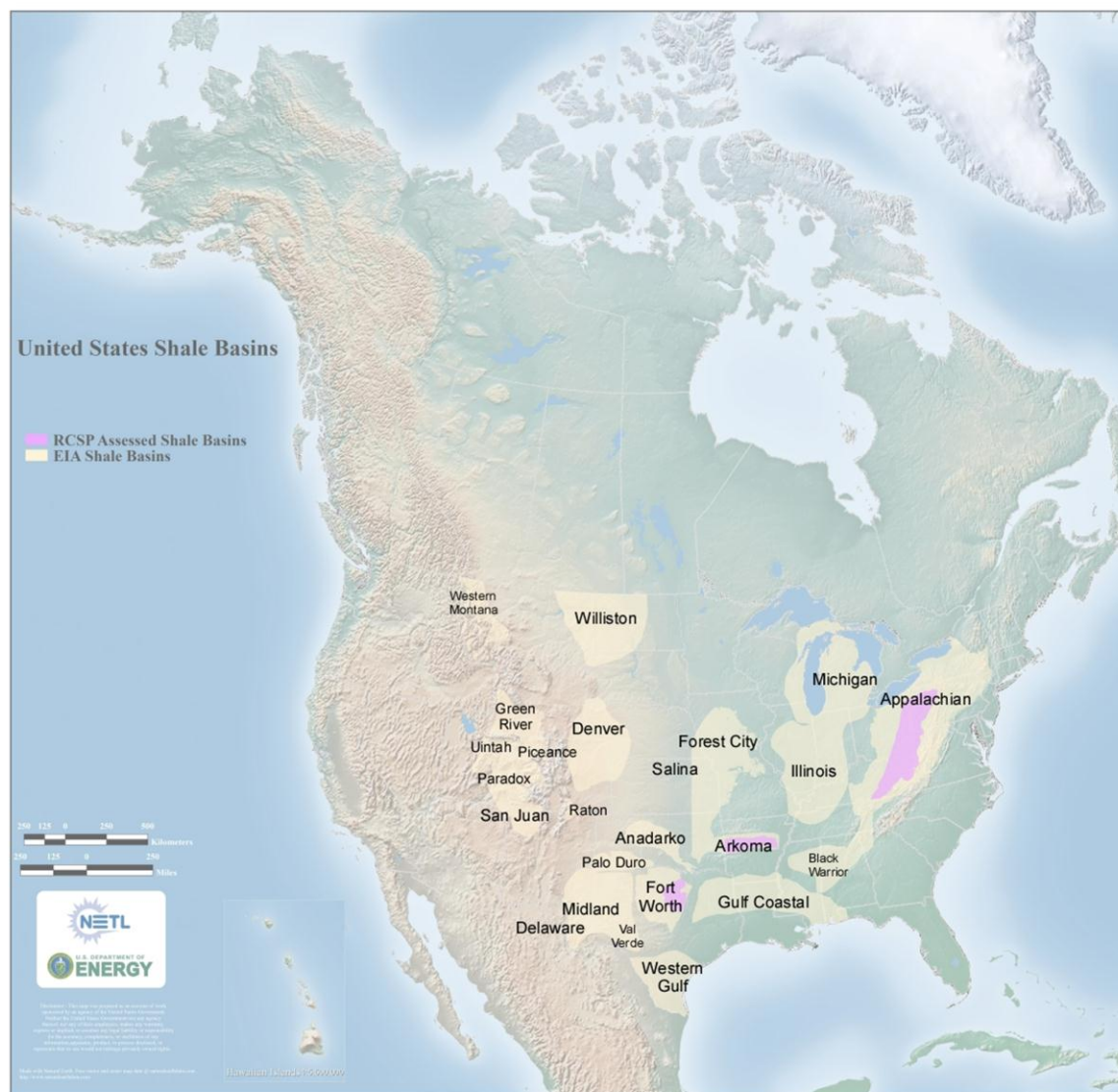
Figure 2-2. Organic-rich shale basins of the United States (from NETL, 2010). Major bedded salt formations are associated with marine shales in many of these basins. Sedimentary basins are the organizing framework for gathering information on individual sedimentary formations for this work package.
