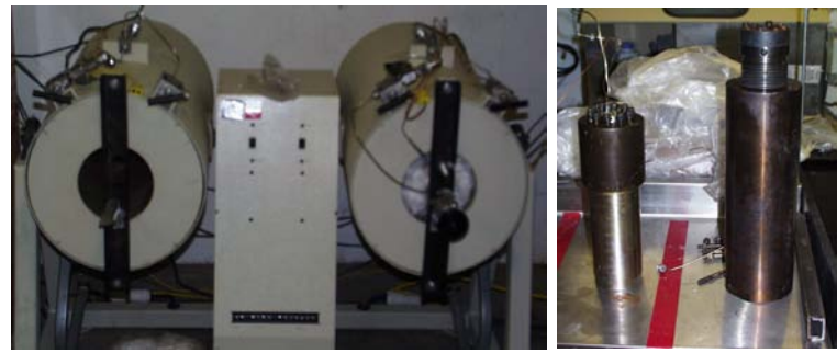
Figure 8. Left: Rocking autoclave rack (400 °C/600 bar) Right: AE (Bridgeman seal-type) pressure vessel, for 600 °C/1.5 kbar furnaces (vessel is ~24" tall).
