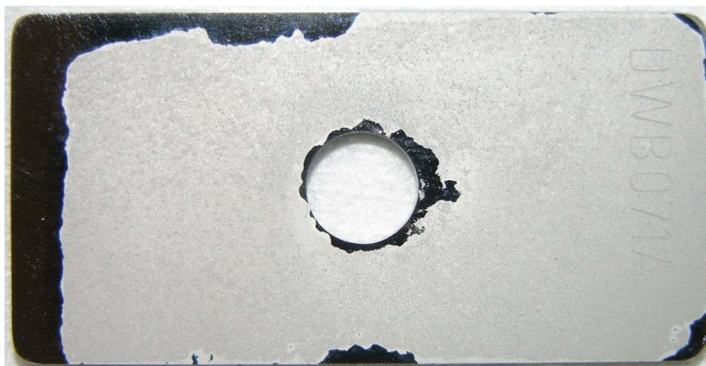
**Figure 11:** Sample DWB071A exposed to SCW at 90°C for 24 months. Dark regions are bare metal, illustrating that the mirror polished surface was unaltered beneath the deposit.
