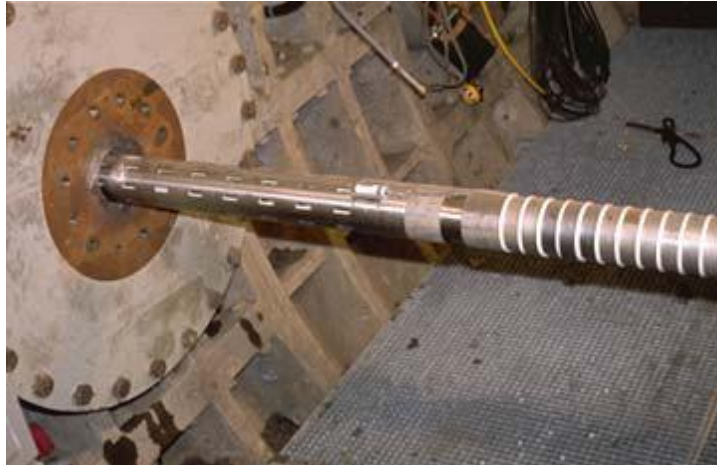
Figure 7. Corrosion testing tube, being prepared for insertion into a test borehole in the Boom Clay formation
