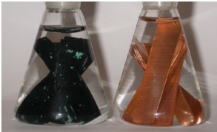
Figure 1. Copper samples immersed in water in a glass container for 15 years. In the container on the left, hydrogen is allowed to diffuse from the bottle through a palladium membrane. The container on the right is completely sealed with platinum
