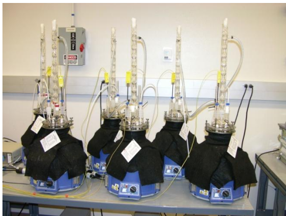
Figure 41. Experimental configuration for long term corrosion performance testing, and polytetrafluoroethylene (Teflon®) sample racks used to suspend coupons within each container
