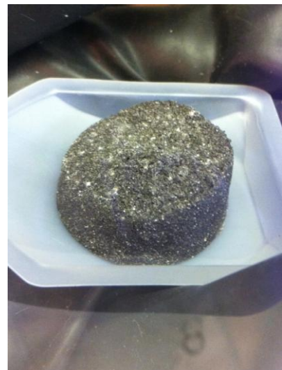
Figure 9. Photograph of glass bonded sodalite ceramic waste form sample containing 10 wt% surrogate ER salt
