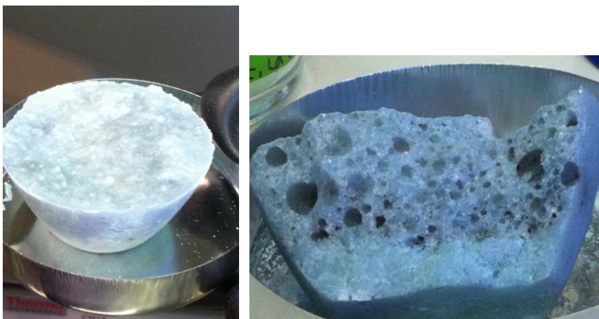
Figure 2. Photographs of surrogate electrorefining salt prior to grinding and sieving.
