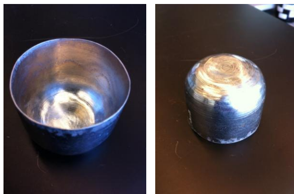
Figure 3. Photographs of platinum crucible used for tellurite glass melting.
