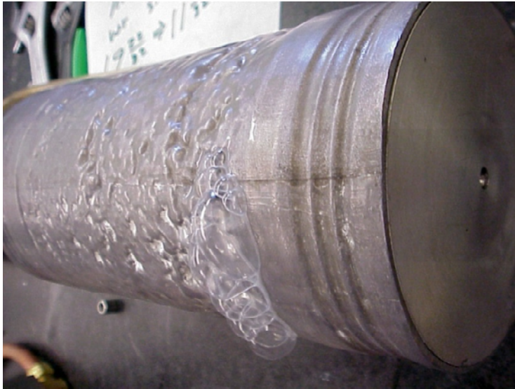
Figure 4 Post-test leak check.
