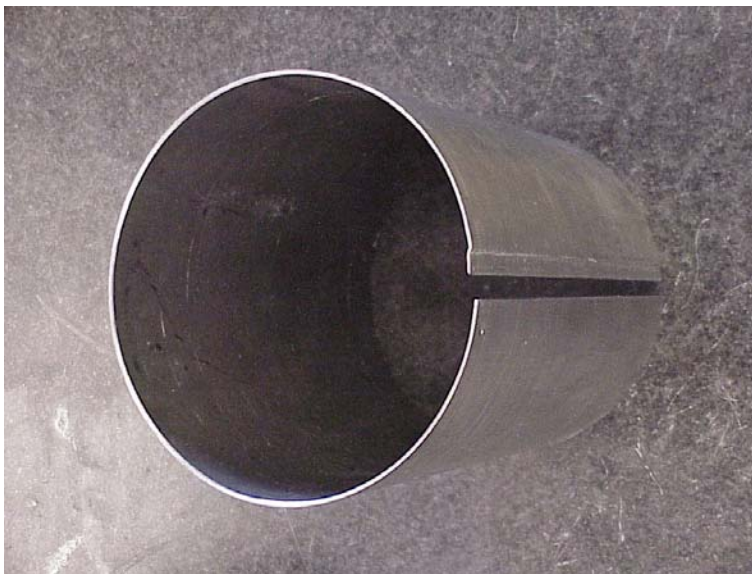
Figure 5 Inner liner showing overlapping joint.
