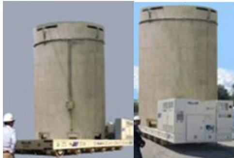
Figure 5-2 Self Propelled Modular Transporter (SPMT) Carrying a UNF Storage Cask
