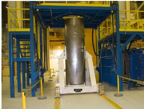
Figure 5-1 Small Transportation Cask on a Small Rail Mounted Cask Transfer Shuttle
