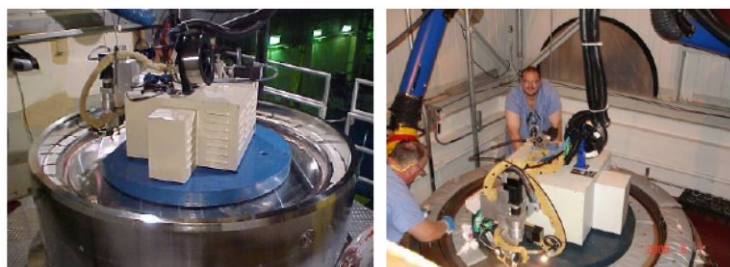
Figure 5-4 Images of Automated Welding System Mounted on Fuel Canister (Reproduced courtesy of Areva Transnuclear)
