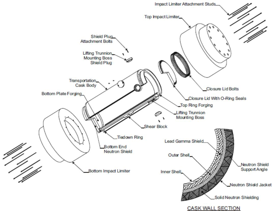
Figure 3-8 Expanded Cutaway View of FuelSolutions TS125 Transportation Package<sup>15</sup>
