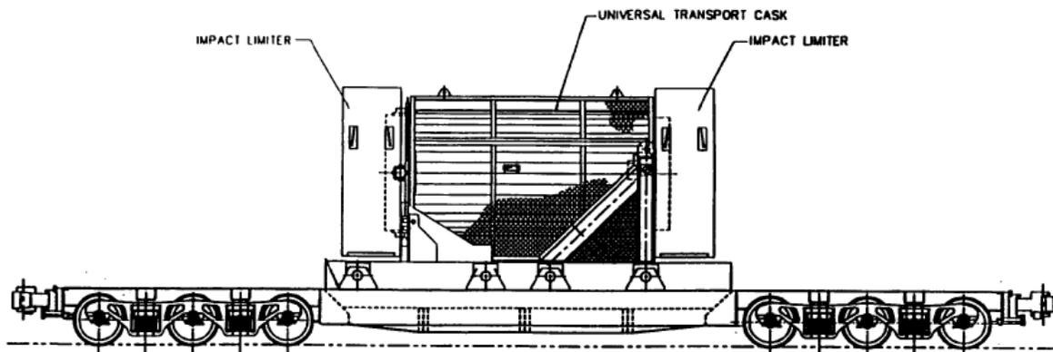
Figure 3-7 NAC-UMS on heavy haul rolling stock
