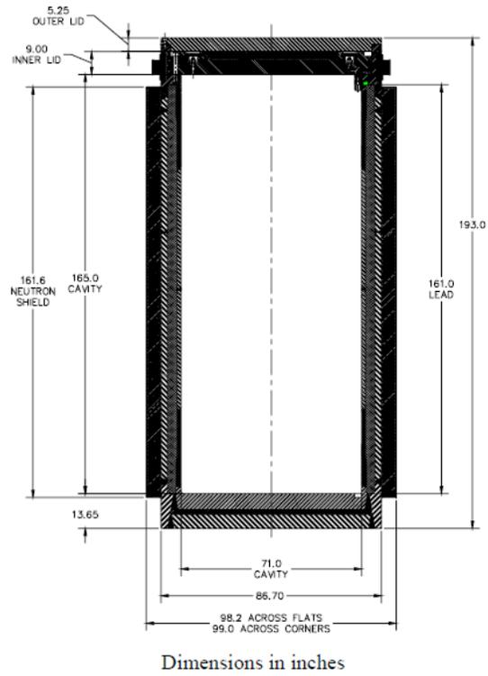
Figure 3-5 NAC-STC Basic Cask Dimensions<sup>13</sup>
