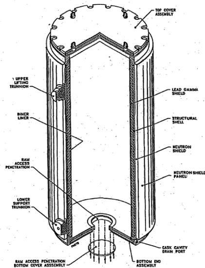
Figure 5-6 OS187H On-Site Transfer Cask<sup>27</sup>
