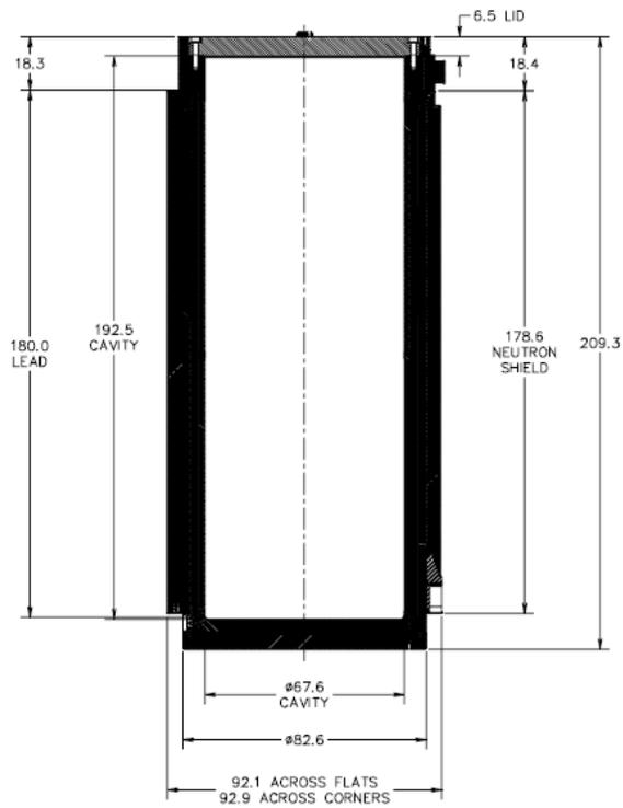
Figure 3-6 NAC-UMS Basic Cask Dimensions<sup>14</sup>
