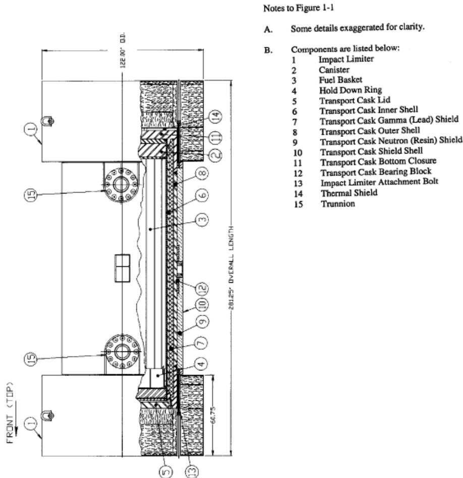
Figure 3-2 NUHOMS MP197 Cask Components<sup>10</sup>
