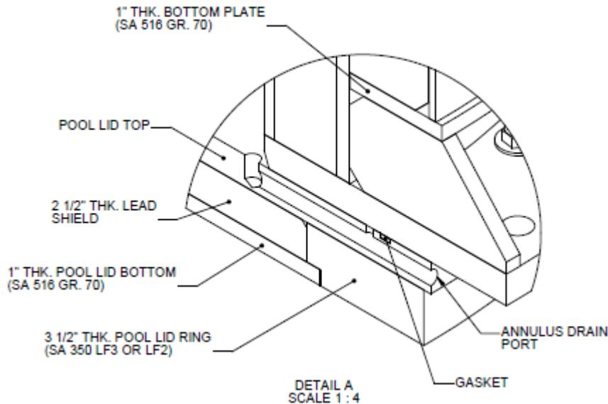
Figure 5-5 HI-TRAC 125D Lower Assembly Detail<sup>25,26</sup>
