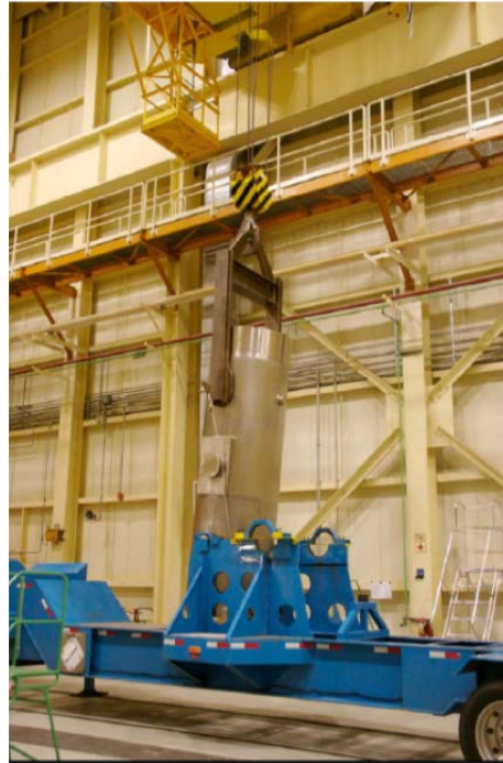
Figure 5-17 A Transportation Cask Is Rotated to A Vertical Position For Placement On A Cask Transfer Car
