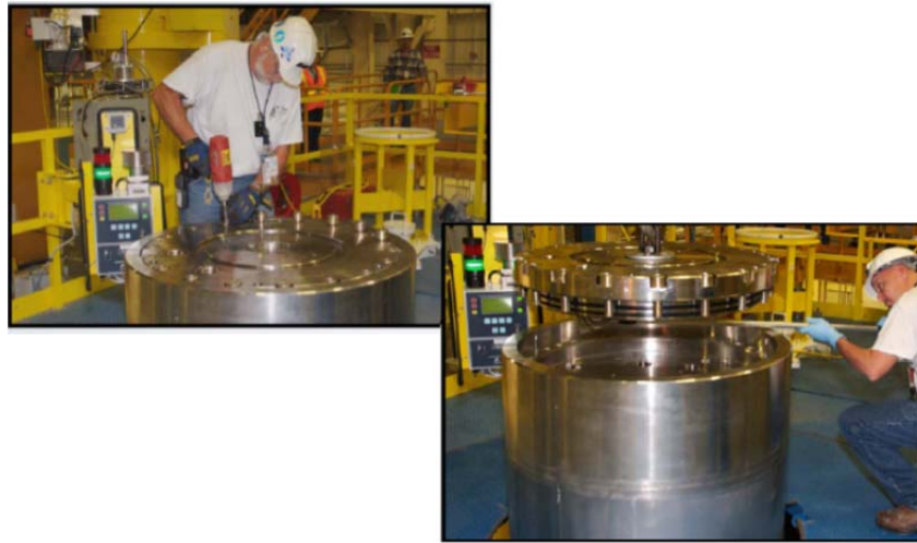
Figure 5-19 Transportation Cask Lid Bolts are Loosened And Radiological Surveys Are Performed Above The Inner Cask Lid
