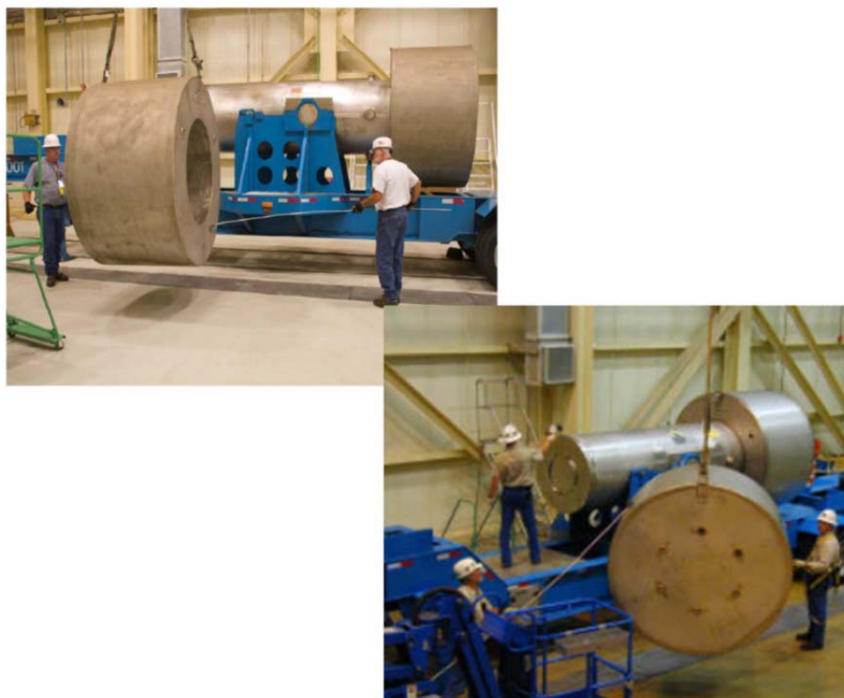
Figure 5-16 Impact Limiters Are Removed From A Transportation Cask
