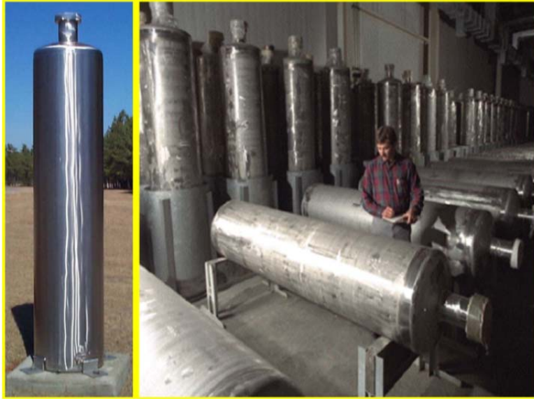
Figure 3-2 SRS HLW Canister And Canisters Being Received (prior to filling with radioactive glass)
