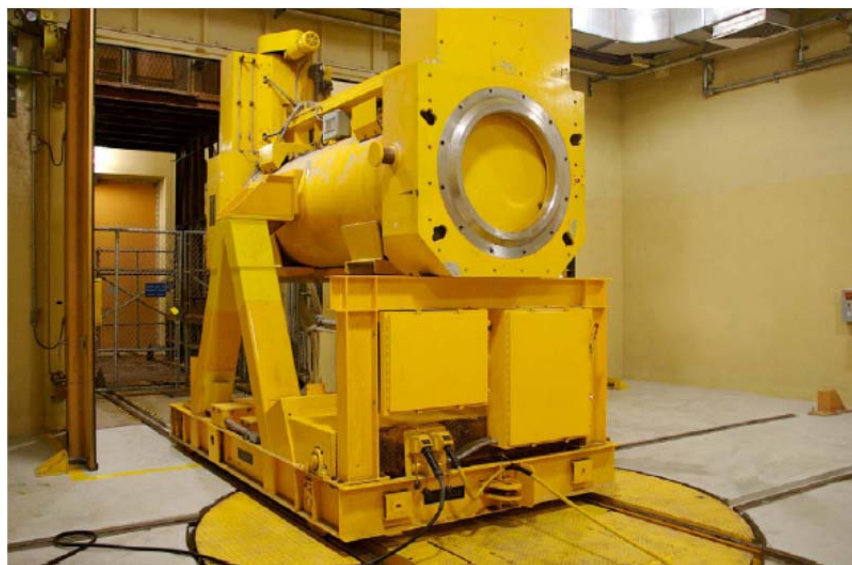
Figure 5-24 The Loaded Facility Cask Is Moved Onto The Waste Shaft Hoist Conveyance For Transfer To The Underground
