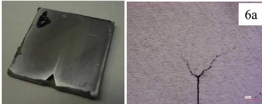
Figure 6: Photos of the sliced SCC specimen. Sample 6a shown in close up of the crack tip.
