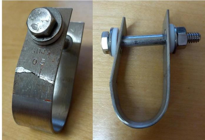
Figure 1: Stress corrosion cracking damage of a Type 304 stainless steel U-Bend sample. Test conditions: T = 95°C, aqueous 42 wt% magnesium chloride solution, time to failure was 89 hours.
