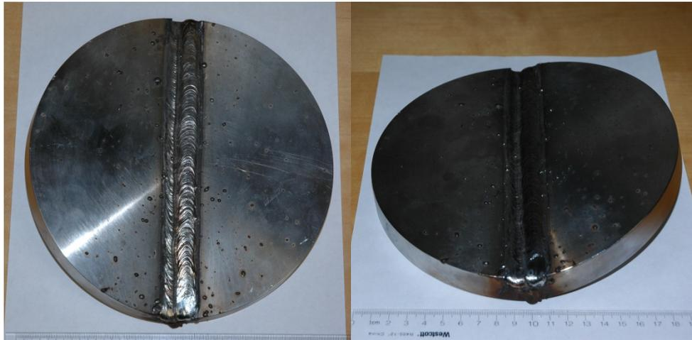
Figure 2: Type 304L stainless steel welded disk for SCC damage tests.
