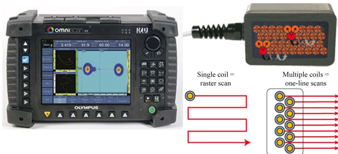
Figure 4.30. Off-the-Shelf Eddy Current Instrument and Probe Array (courtesy of Olympus NDT)
