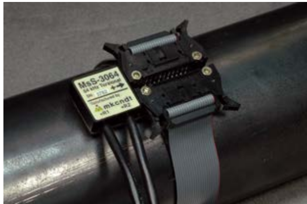
Figure 4.46. Photograph of Ribbon Cable MsS Transducer for Axial Pipe Inspections (photo courtesy of Guided Wave Analysis LLC)
