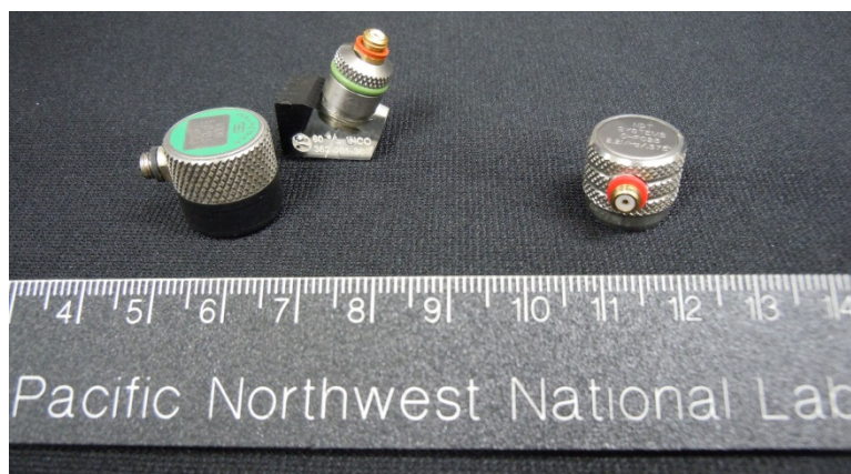
Figure 4.16. Several 2.25-MHz and 5.0-MHz Contact Ultrasonic Transducers Including a Transducer Mounted to a Wedge for Angle-Beam Inspections
