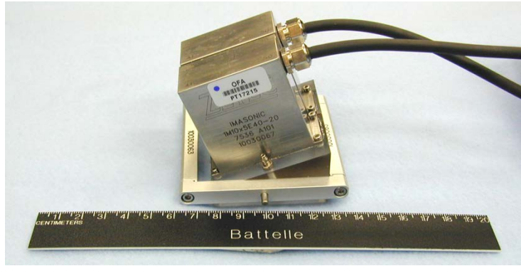
Figure 4.17. A 1.0-MHz Phased-Array Probe Consisting of a Transmitter and Receiver Unit
