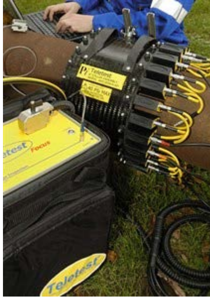
Figure 4.44. Photograph of the Teletest Focus Plus Inflatable Ring Transducer. Reproduced courtesy of Plant Integrity Ltd. (a TWI subsidiary company)
