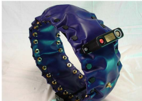
Figure 4.45. Photograph of Inflatable Ring Transducer. Image used with permission of Guided Ultrasonics Ltd.
