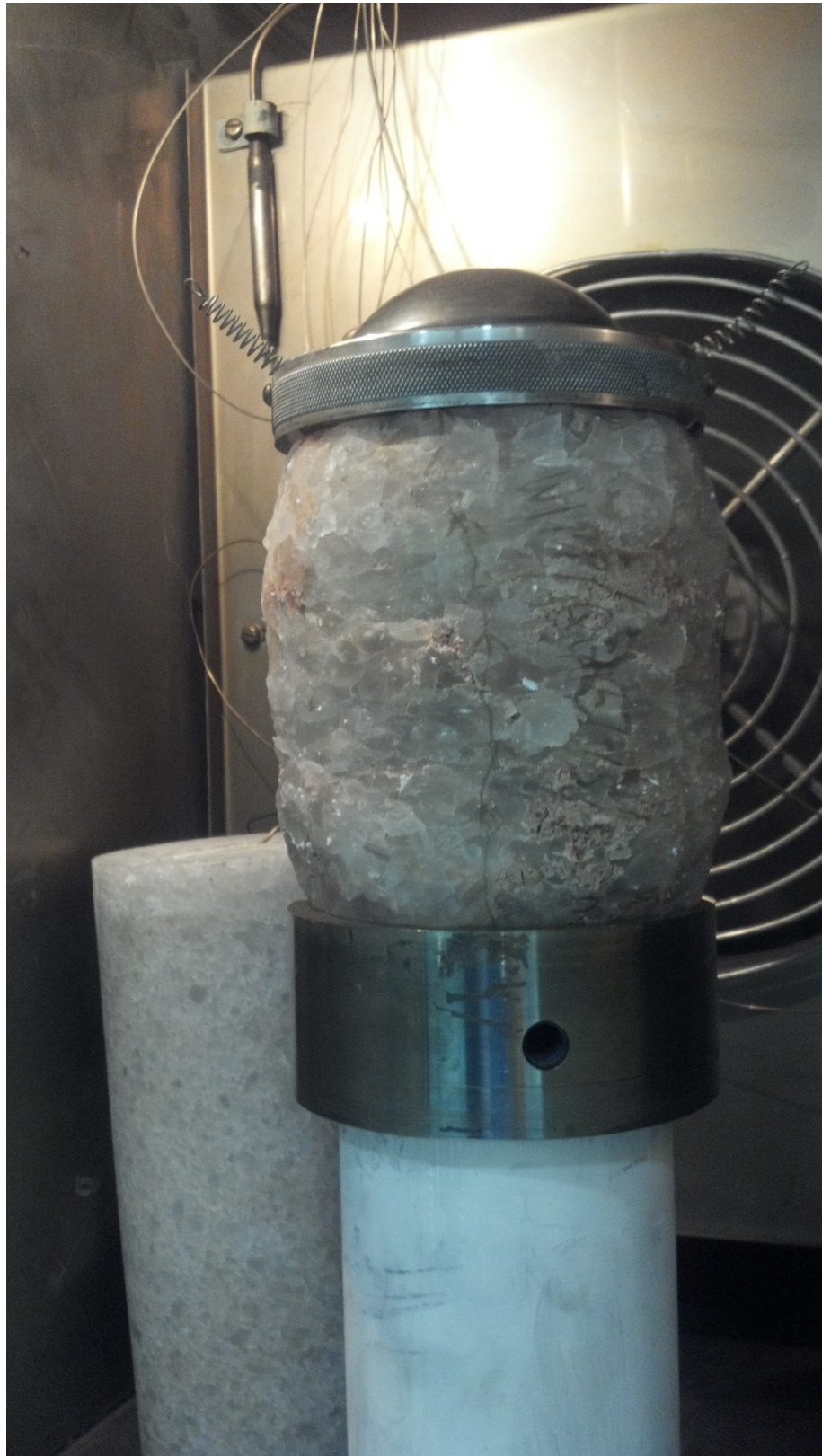
Figure 14. Posttest Photograph of Specimen WIPP/QGU37-15/1 Tested at 250°C.
