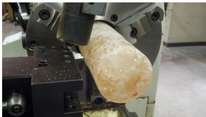
Fig. 1. Typical horizontal lathe machining setup for preparing cylindrical specimens.
