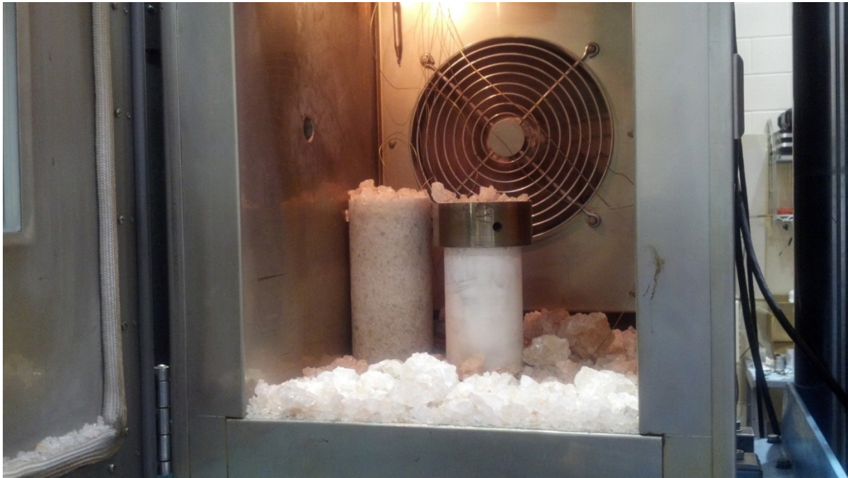
Figure 8. Posttest Photograph of Specimen WIPP/QGU37-20/2 Rubble.
