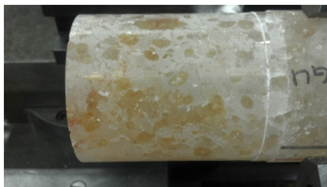
Fig. 2. Waste Isolation Pilot Plant salt specimen brine inclusions (darker ovoid areas are wet).
