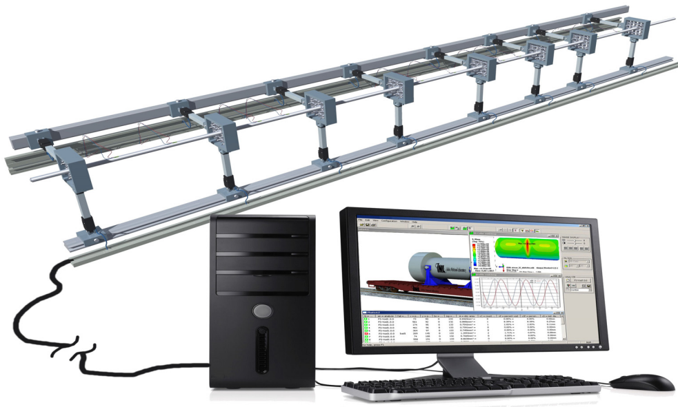
Figure 2.1-3: Conceptual hybrid test set-up for experimental testing of high burnup fuel rod (note the rod would be in a hot-cell). This test configuration simulates the package in Figure 2.1-2.
