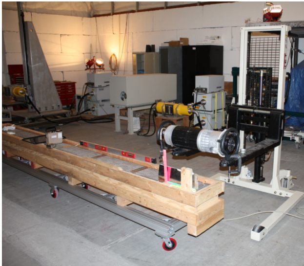
Figure 4.1-1: X-ray scanning setup for NDE tests
