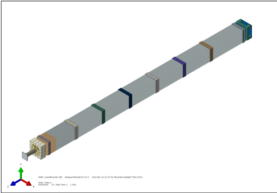
Figure 3.1-6. Model of the Westinghouse PWR 17 x 17 assembly created in Abaqus 6.12-2 (converted from the LS-DYNA model documented in Adkins ).
