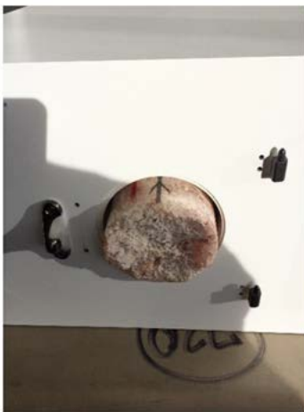
Figure 3. Picture showing a salt core in the measurement cavity of a Corona low-field NMR instrument.
