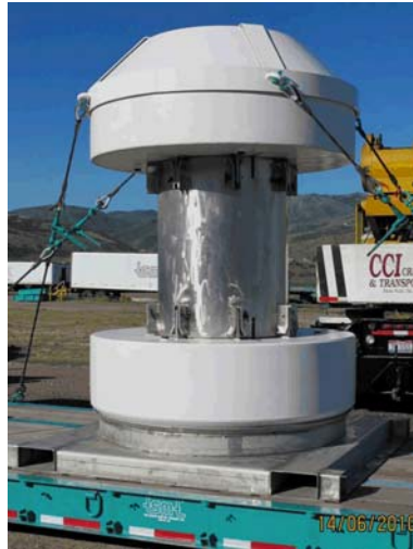
Figure 2.1. BEA Research Reactor Cask (printed with permission from AREVA Federal Services)
