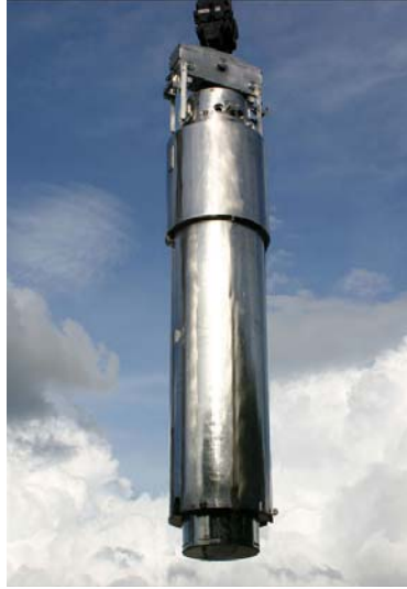
Figure 2.2. NAC LWT Shipping Cask (printed with permission from NAC International)
