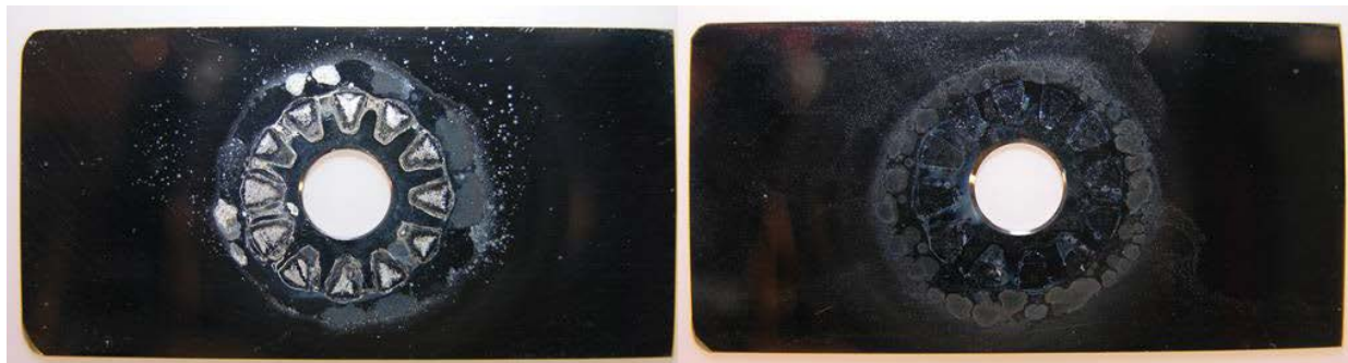
Figure 38. 304SS coupon with 200 \mu\text{g}/\text{cm}^2 and 7 day exposure after crevice former removal (L) and rinsing (R).
