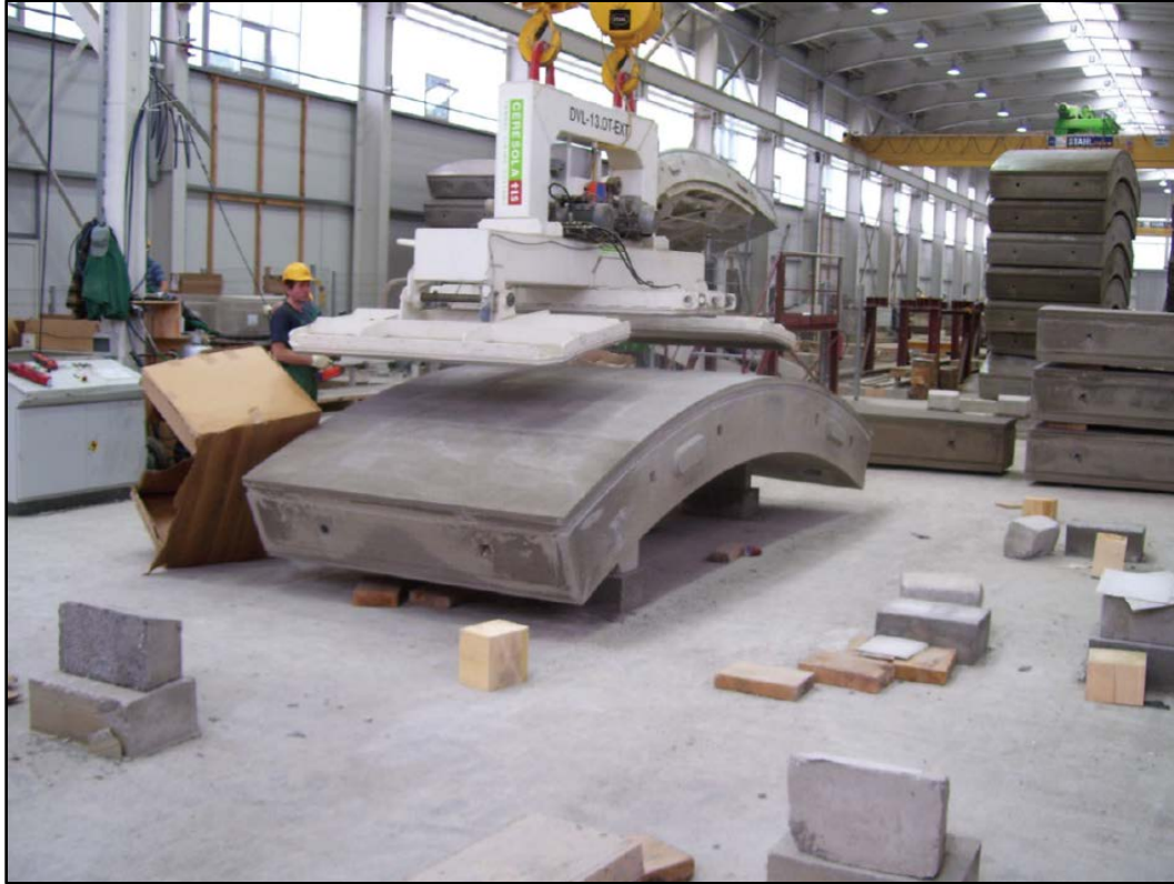
Figure 4. Pre-cast reinforced concrete liner segment, removal from forms, for a single-pass liner (Hung et al. 2009, Figure 10-7).
