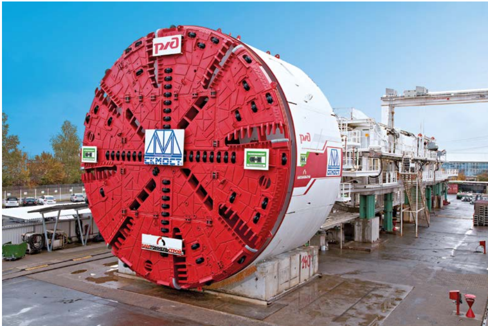
Figure 2. Open-type single-shield TBM with trailing gear, during assembly, Russian road tunnel project (13.2 m diameter) ( www.herrenknecht.com ).
