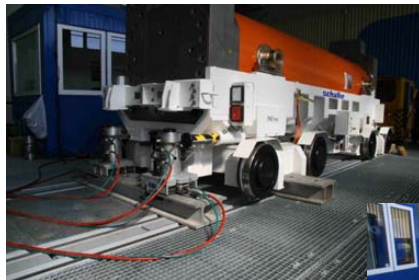
Re-railing of transport cart loaded with transfer cask using standardized equipment (Deutsche Bahn)
