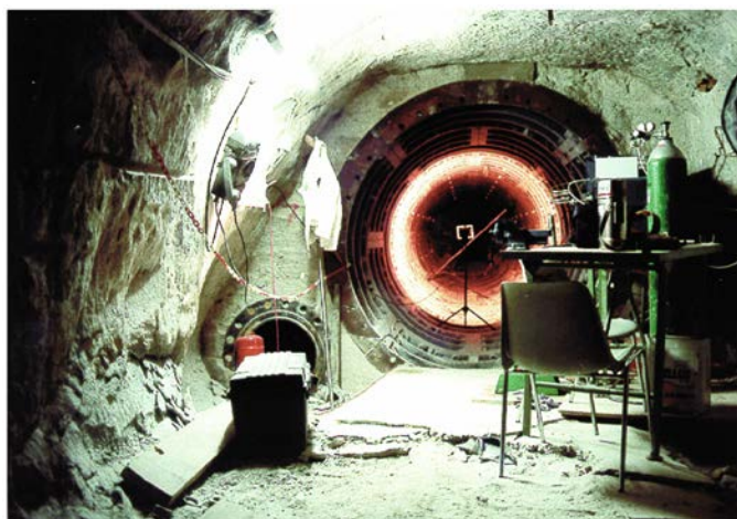
Figure 2. Joint Project models this liner configuration in the Asse Mine.
