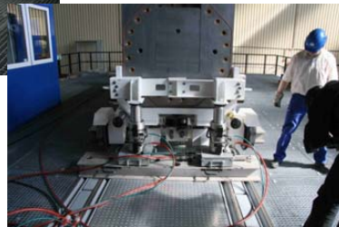
Re-railing of transport cart loaded with transfer cask using standardized equipment (Deutsche Bahn)
