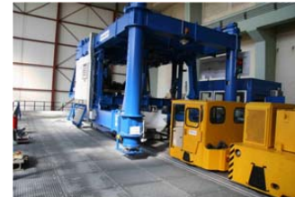
Emplacement machine towing with the transport cart and the locomotive
