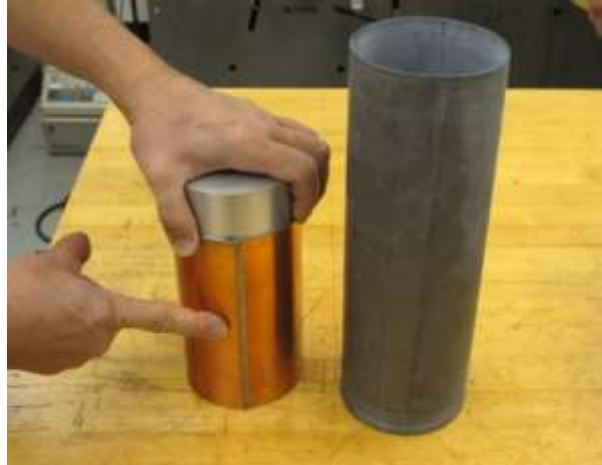
Figure 5a. Application of Copper Jacket.
