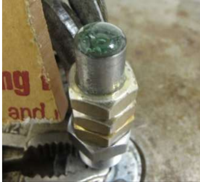
Figure 6. Brine exiting the pore pressure port at 250°C.
