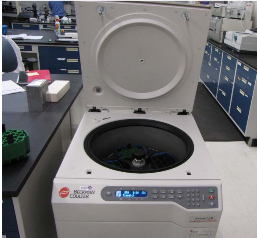
Figure 2. The centrifuge to be used in capillary pressure and relative permeability tests.
